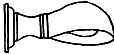
Suitable Lighting Above the Kitchen Sink. A frosted bulb used in this type of globe produces a soft light without glare, which is highly desirable.
