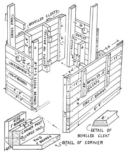
Fig. 2.—Perspective drawing showing how the form is made. The dimension: on this drawing are for a tank the proper capacity for six persons.
