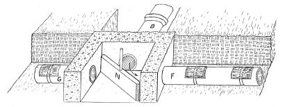
Fig. 7.—Detail drawing of the distributing box. This view shows how the valve is made and used to deflect incoming liquid first to one distributing tile line, then to the other. The tile line B, from the tank to the box, is made of four-inch sewer tile with cemented joints. G and F show the two distributing tile lines. They are four-inch drain tile laid with loose joints about 1/8 inch apart and the top half of the joint is covered with tar paper.
