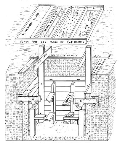
Fig. 5.—A Cross-sectional view showing how the tank appears after the concrete has been put in and before the forms are removed. The method of bracing and the method of holding the inlet and outlet tiles in place are clearly shown. At the top of the picture is shown how the four slabs are made for the cover.
