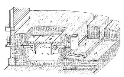
Fig. 1.-Cross Section of Septic Tank and Distribution System.
