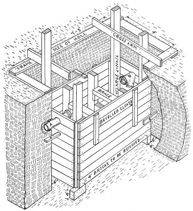
Fig. 3.—This drawing shows the form set in the hole ready for the concrete. The bricks under the corners should be removed before putting in the concrete. The top three end boards are not nailed. (See Fig. 2.)
