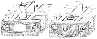
6c.—The hole with the form and and concrete all in place.
