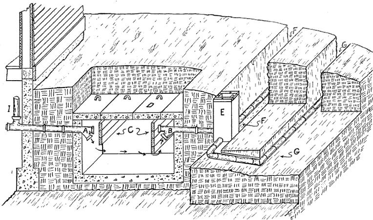
**Fig. 1.—Cross Section of Septic Tank and Distribution System.**
