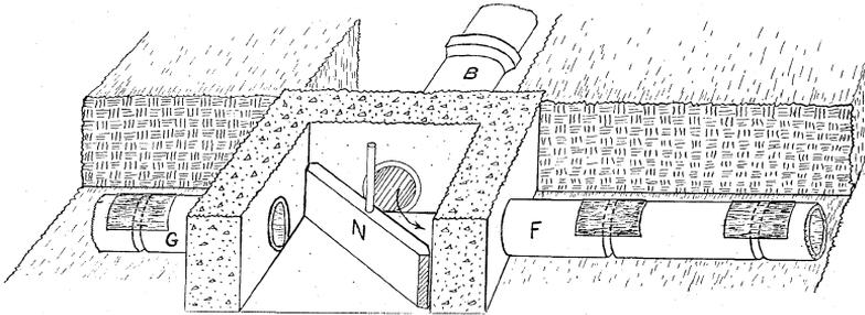
Fig. 7.—Detail drawing of the distributing box. This view shows how the valve is made and used to deflect incoming liquid first to one distributing tile line, then to the other. The tile line B, from the tank to the box, is made of four-inch sewer tile with cemented joints. G and F show the two distributing tile lines. They are four-inch drain tile laid with loose joints about  $1/8$  inch apart and the top half of the joint is covered with tar paper.
