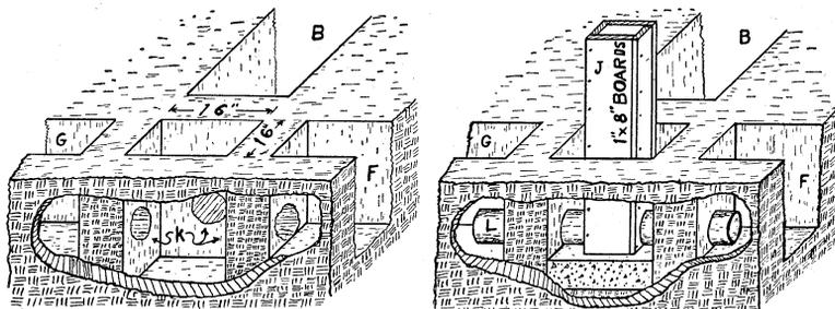
Fig. 6a.—The hole dug ready for the form.
