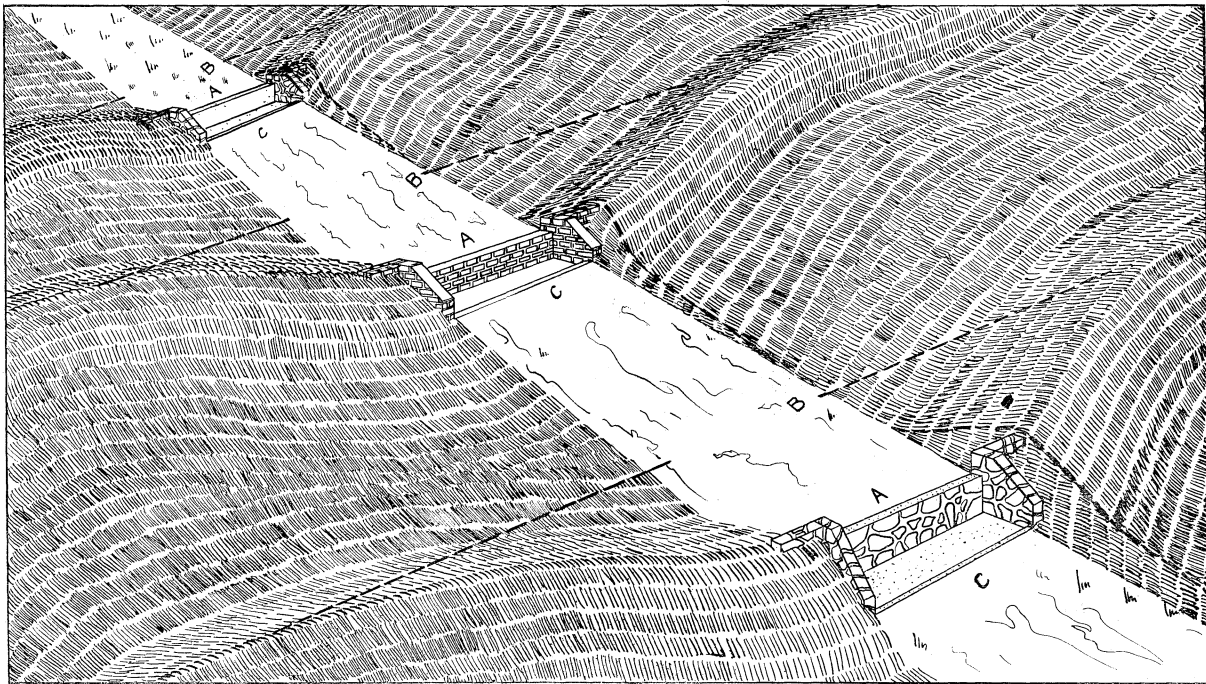
Fig. 1.—Showing how to locate the baffles in the terrace outlet ditch. The baffles, "A," are located one vertical foot below "B," where the terrace lines enter the ditch. The ends of the terraces are shown curved out of their natural course to connect with the baffles. The lower ends are built extra high to make up for the baffles being a foot low. The portion of the ditch above the top baffle is protected by vegetation.
