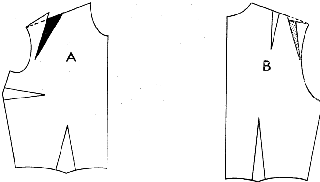
Figure 25a and b—Adjust pattern shoulder length. Example A shows widening the shoulder, Example B narrows the shoulder.
