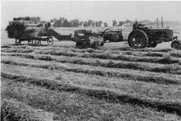
Fig. 9—The modern pickup baler picks up the alfalfa and bales it direct from the windrow.
