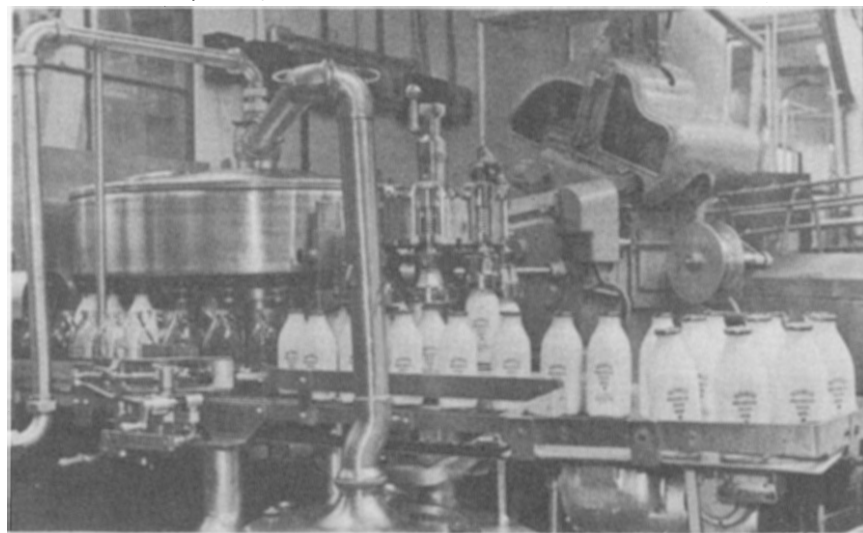
4—Sanitary—Labor saving methods used in bottling fluid milk. Silver Seal Cap Machine and bottle filler in action.
