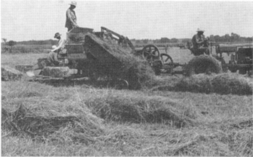
Figure 2. The modern pickup baler picks up the alfalfa and bails it direct from the windrow.
