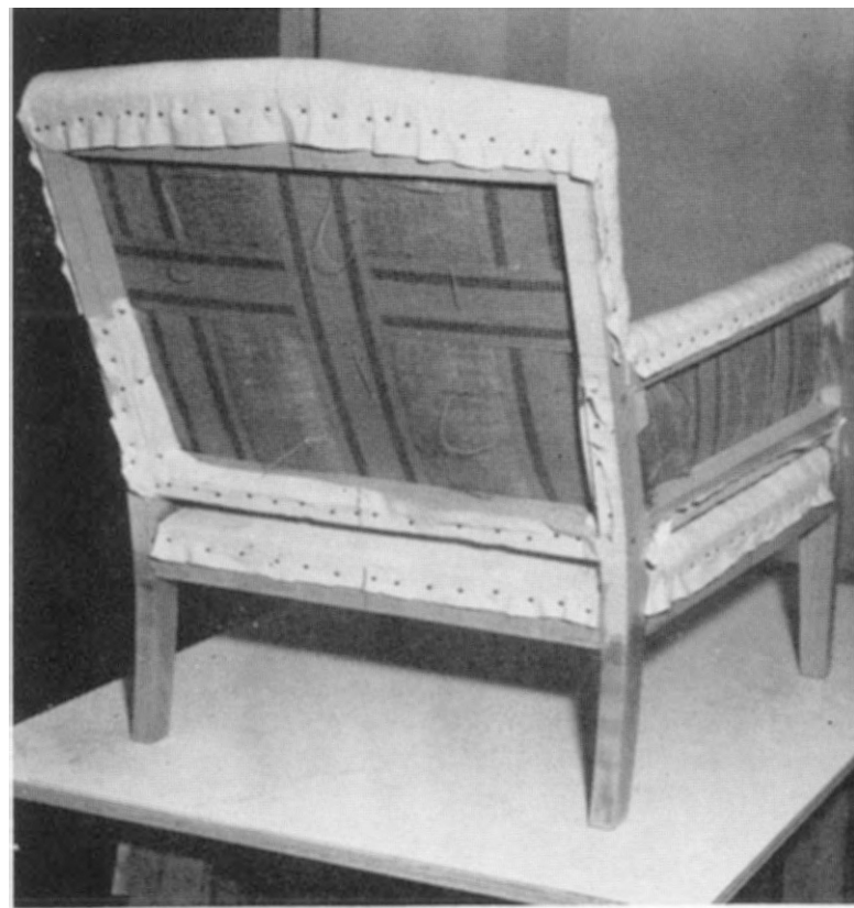
Fig. 34 Chair Ready for Upholstery Fabric—Back View
