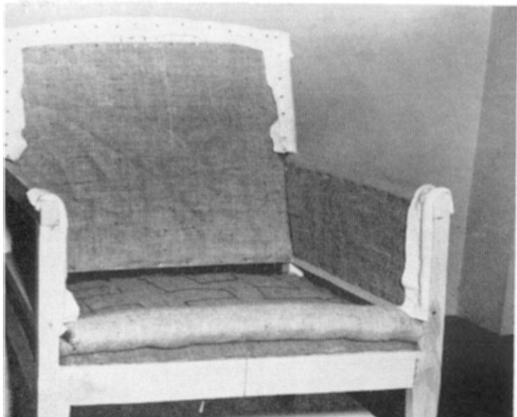
Fig. 25 Completed Edge Roll
