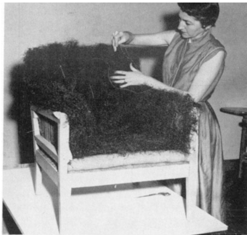
Fig. 26 Sewing Moss into Place with Mattress Twine
