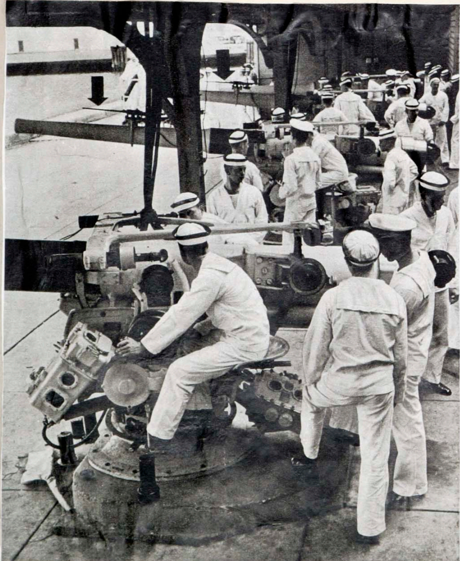
GUN CONTROL is practiced on these 4-inch weapons. Crews do regular sighting, aiming, etc., but practice firing is done by the small gun on the barrel top (arrows).
