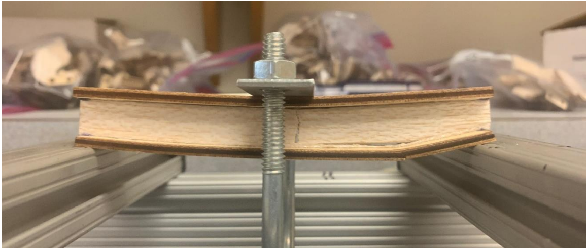
Figure 61: Prototype I-Beam with-grain shear failure
