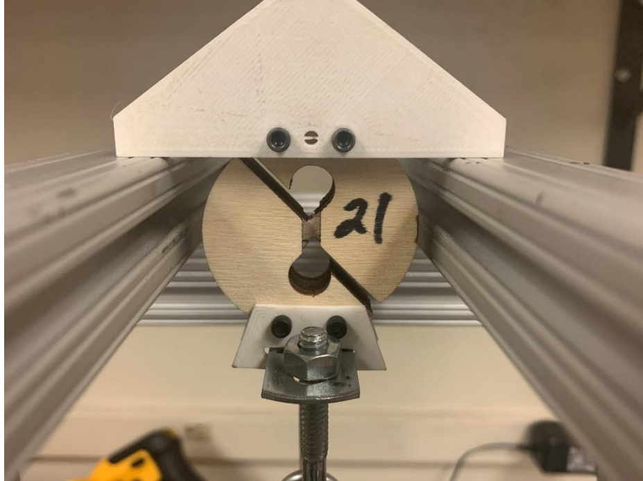
Figure 46: Cross-Grain shear test setup
