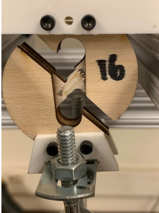
Figure 48: Cross-grain Shear Test Failure
