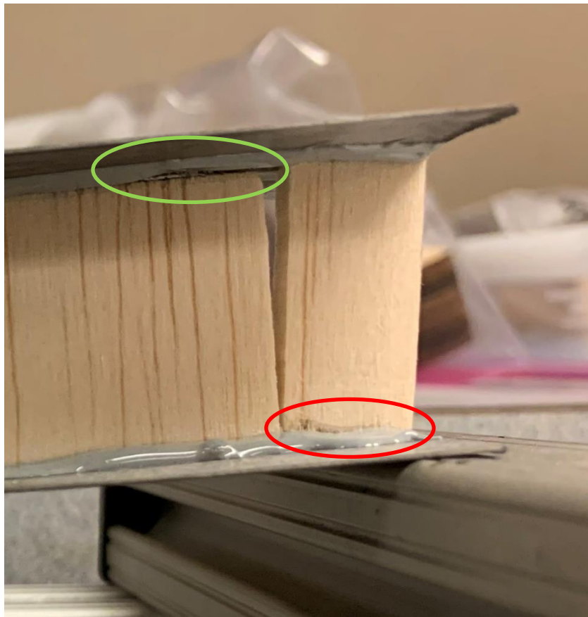
Figure 79: Inspection of Failure in 5" I-Beam
