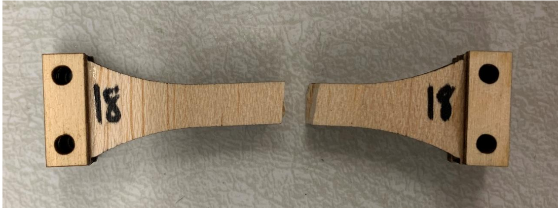
Figure 36: With-grain Tensile Test Failure
