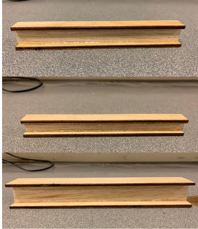
Figure 58: I-beams with plywood caps and with-grain balsa wood shear webs
