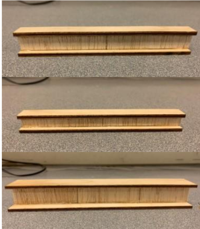
Figure 57: I-beams with plywood caps and cross-grain balsa wood shear webs
