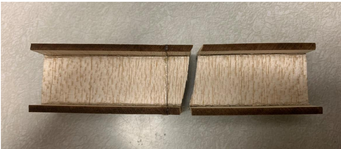
Figure 62: Prototype I-Beam tensile failure
