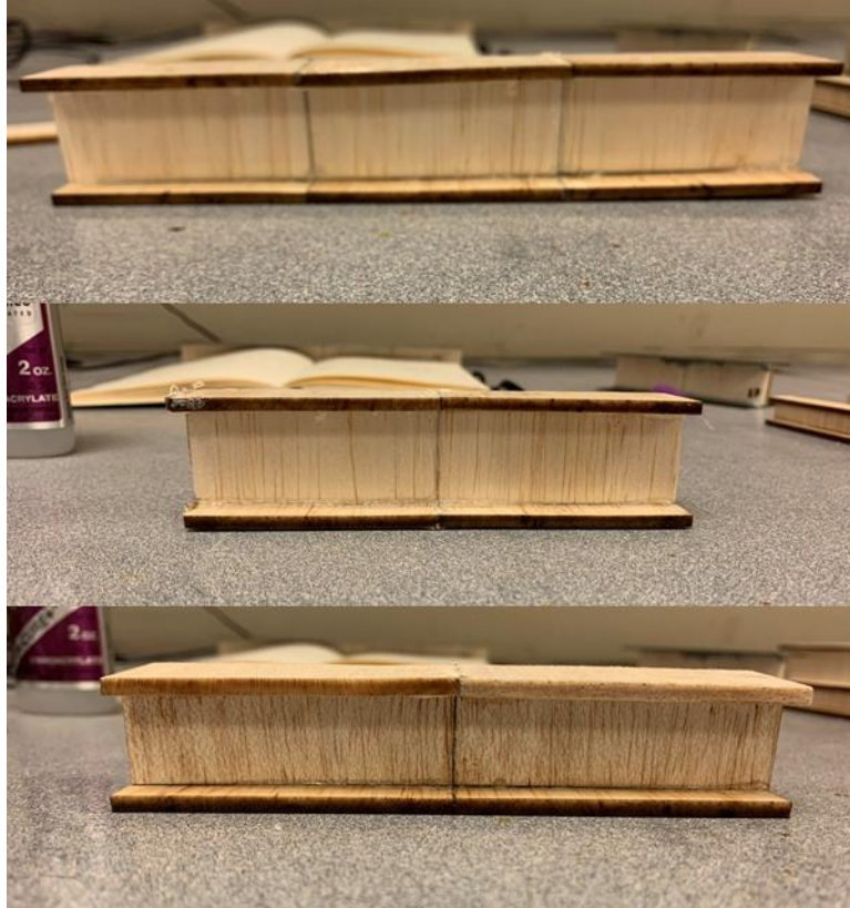
Figure 59: I-beams with with-grain balsa wood caps and cross-grain balsa wood shear webs
