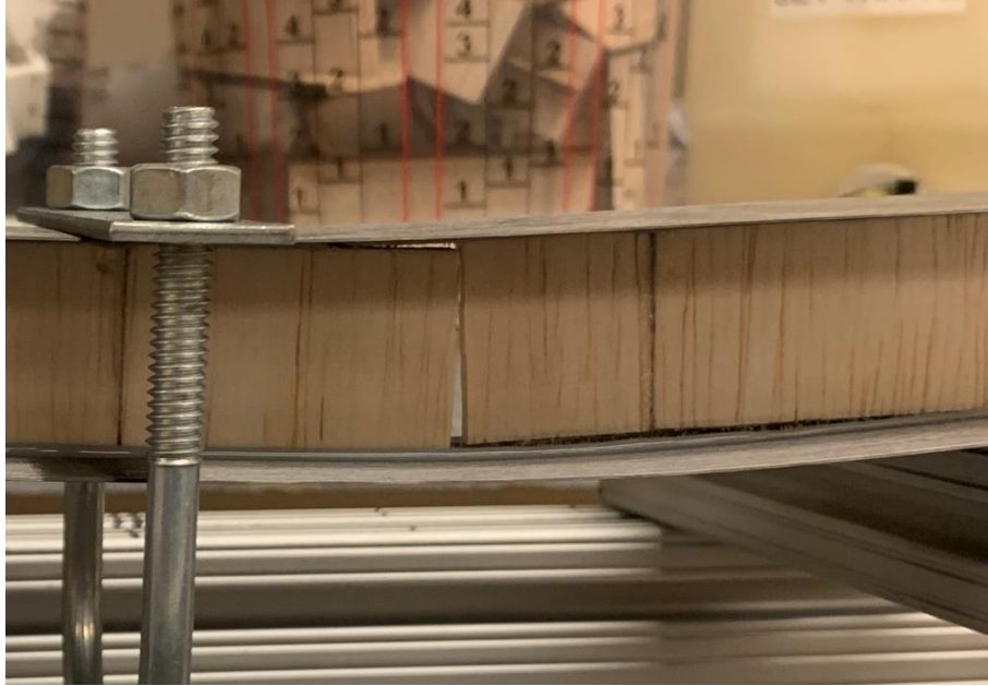
Figure 81: Failure of 10" - Sample 3 Composite I-Beam
