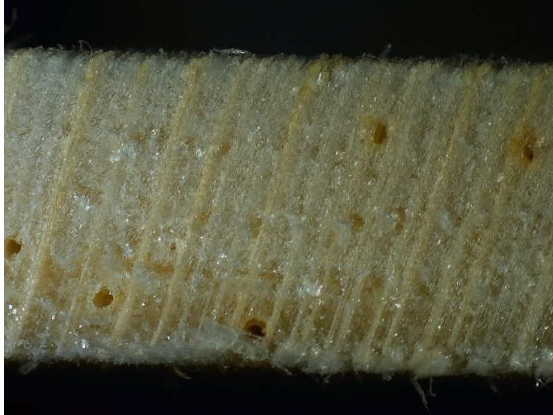
Figure 13: Cross-grain of balsa wood cellular makeup
