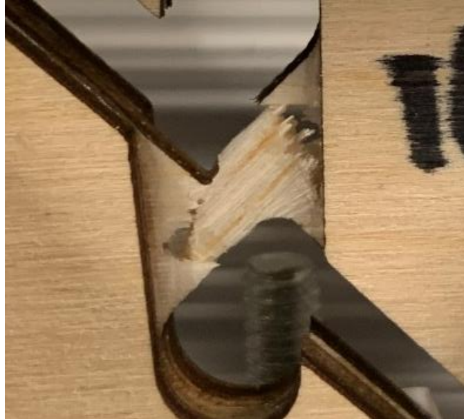
Figure 51: Complete failure of shear test sample
