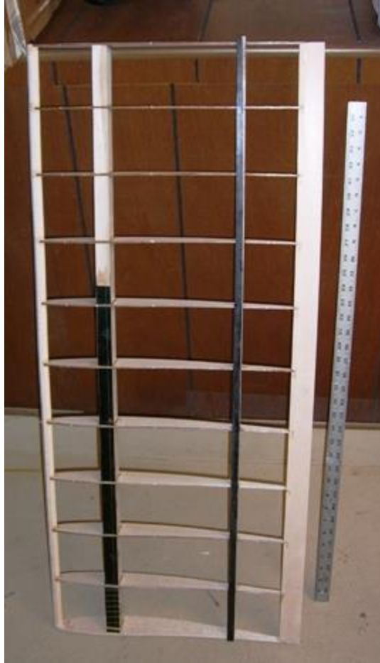
Figure 5: RC airplane wing using carbon fiber caps, spruce, and balsa wood
