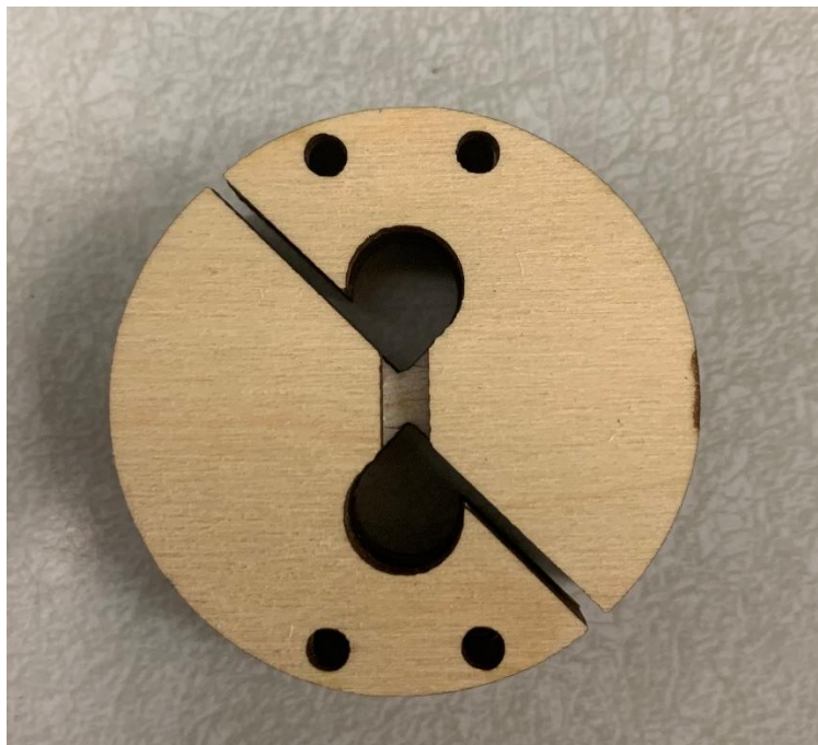
Figure 45: Physical cross-grain shear test sample
