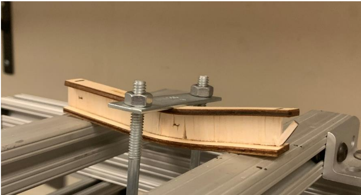
Figure 60: Prototype I-Beam cross-grain shear failure
