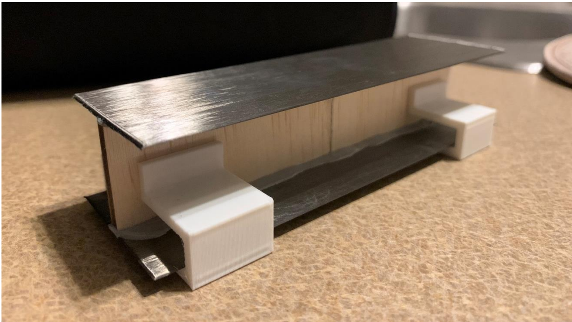
Figure 75: Composite I-beam manufacturing with 3D-printed jigs
