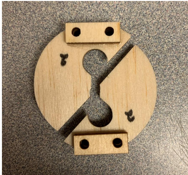
Figure 47: With-grain Shear Test Failure
