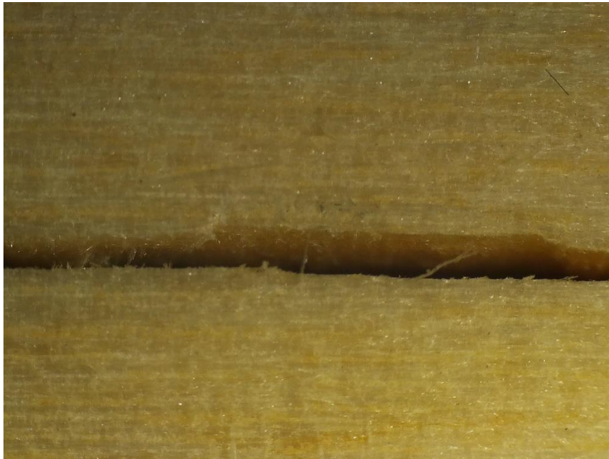
Figure 82: View of 10" - Sample 3 I-Beam Failure Under Microscope
