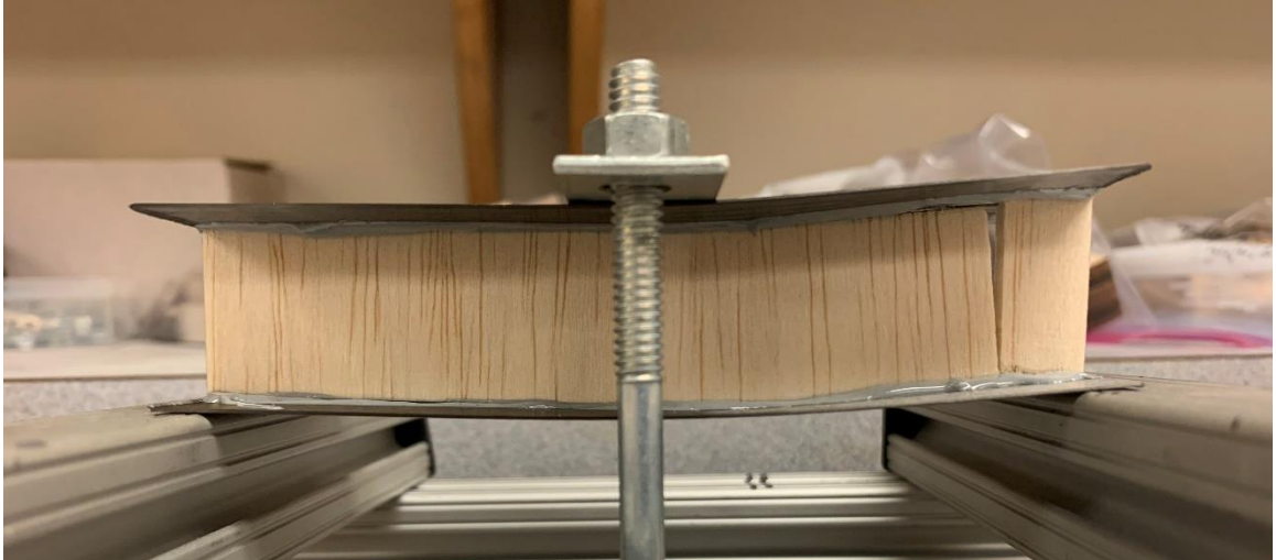
Figure 76: 5" Composite I-Beam Failure
