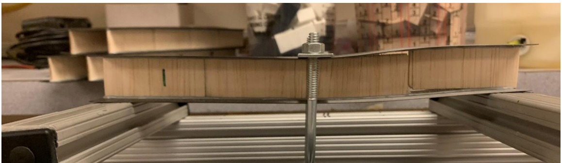
Figure 78: 10" Composite I-Beam Failure
