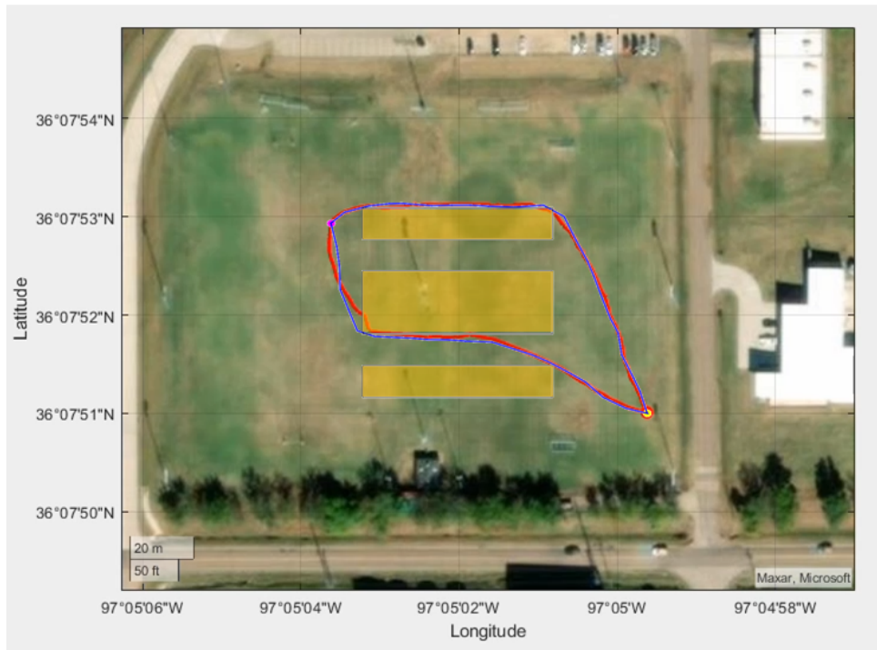
Figure 89: The first Eagle Test with multiple rectangular obstacles
