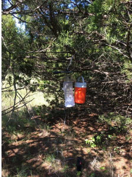
Fig 1. CDC Light trap, without light, baited with two pounds of dry ice in ERC.
