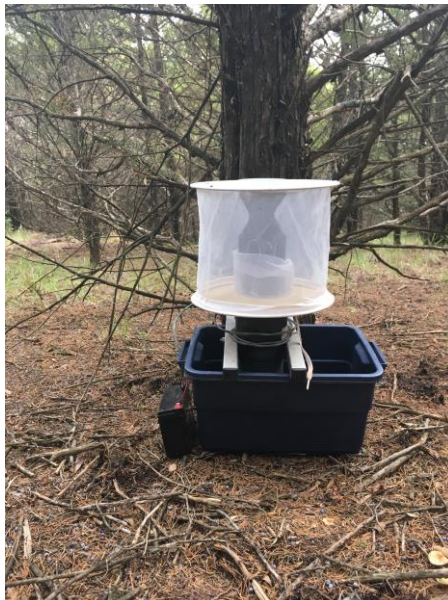
Fig 2. Gravid trap baited with fermented grass water in ERC.
