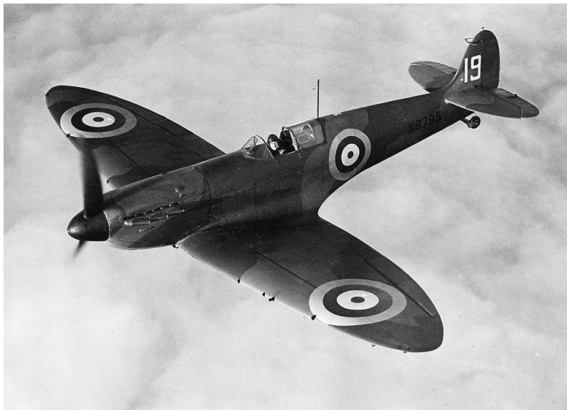
Figure 1: the Supermarine Spitfire, 9th Production Mk I (1938), which created an elliptical span loading through its unique planform shape
