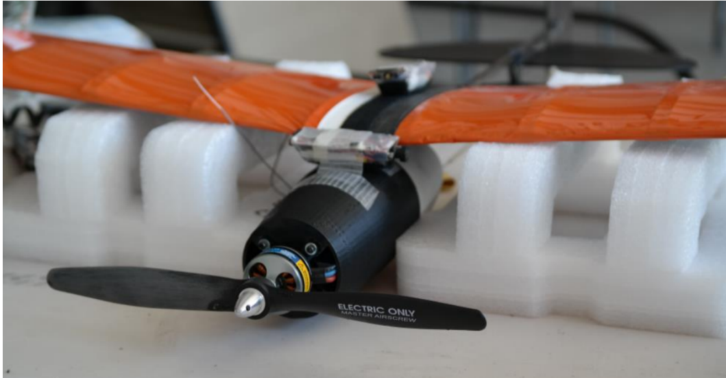
Figure 76: Christopher Banfield's 3D printed aircraft, with 3D printed ribs and a monokote-style covering
