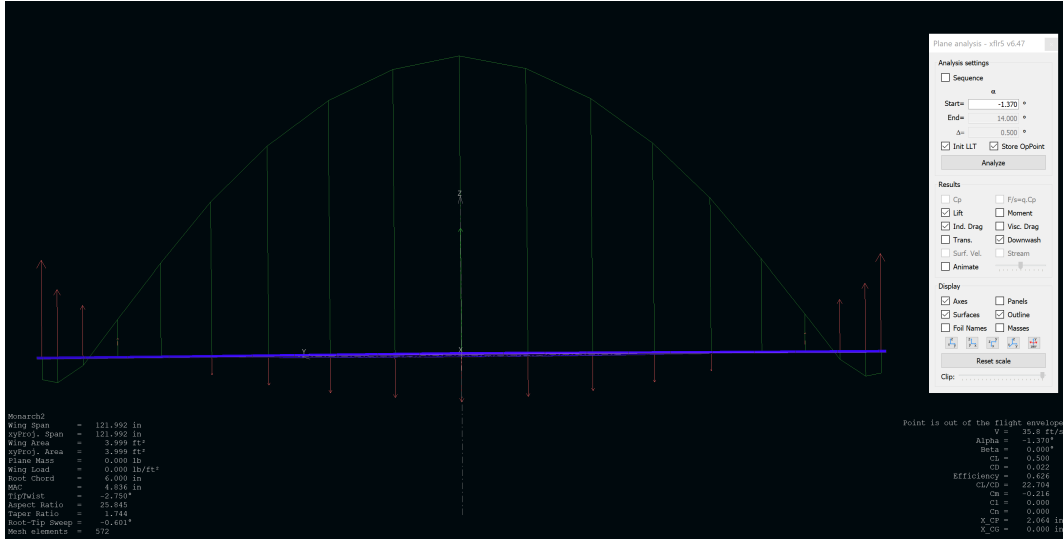
Figure 59: LLT Results in XFLR5 for STCA
