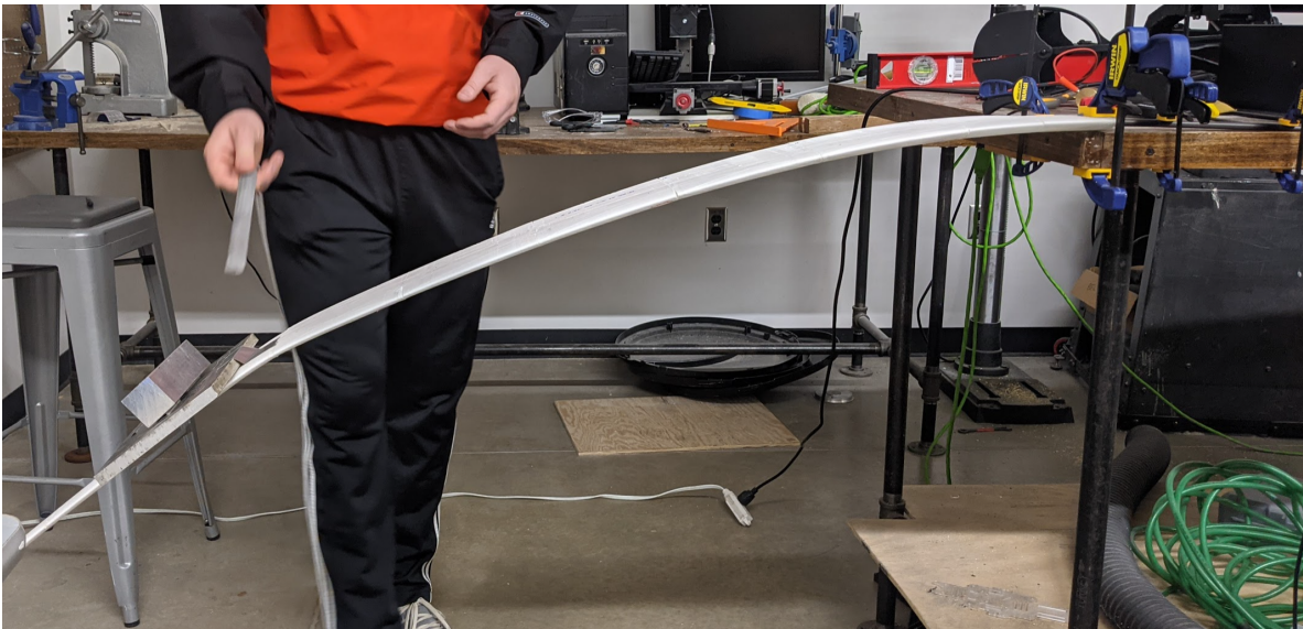
Figure 84: Max Loading on 3D printed Wing before Yielding: 5.7 lbs 40 inches from root
