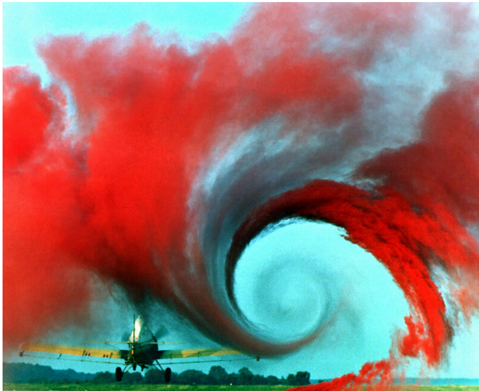
Figure 20: Wing's trailing vortex, visualized through red smoke
