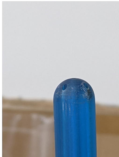
(b) Damaged Probe Tip
