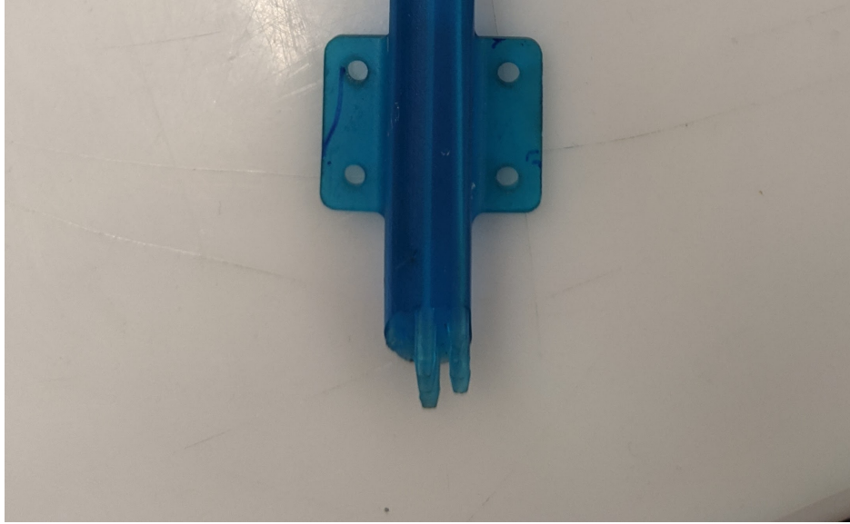
Figure 51: Broken Probe Pitot Attachment
