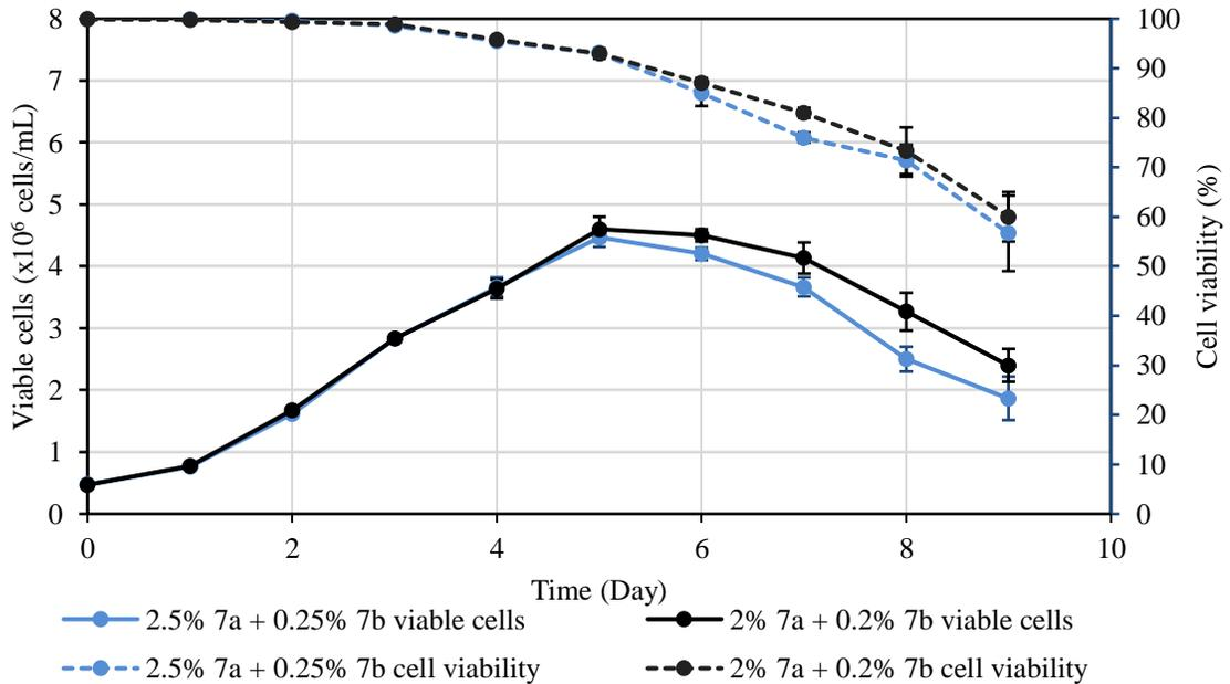
Figure 8. Growth profile for fed-batch culture using Cell boost 7a and 7b starting on day 3 every day.
