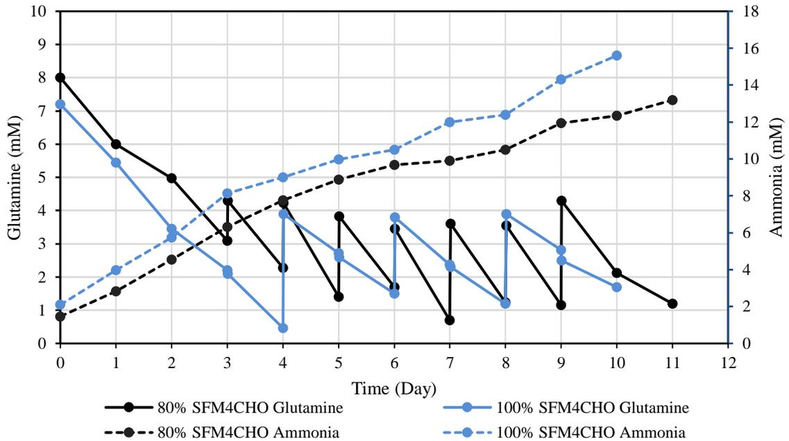
Figure 16. Glutamine and ammonia concentration profile for fed-batch culture using 1.5%:0.1% Cell Boost 7a/7b every other day with 100% and 80% SFM4CHO medium.
