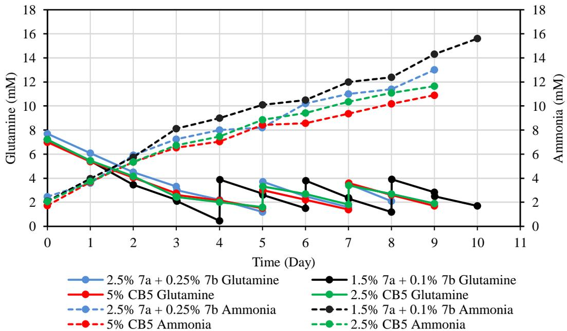
Figure 13. Glutamine and ammonia concentration profile for fed-batch culture using cell supplements 7a/7b or CB5 every other day.
