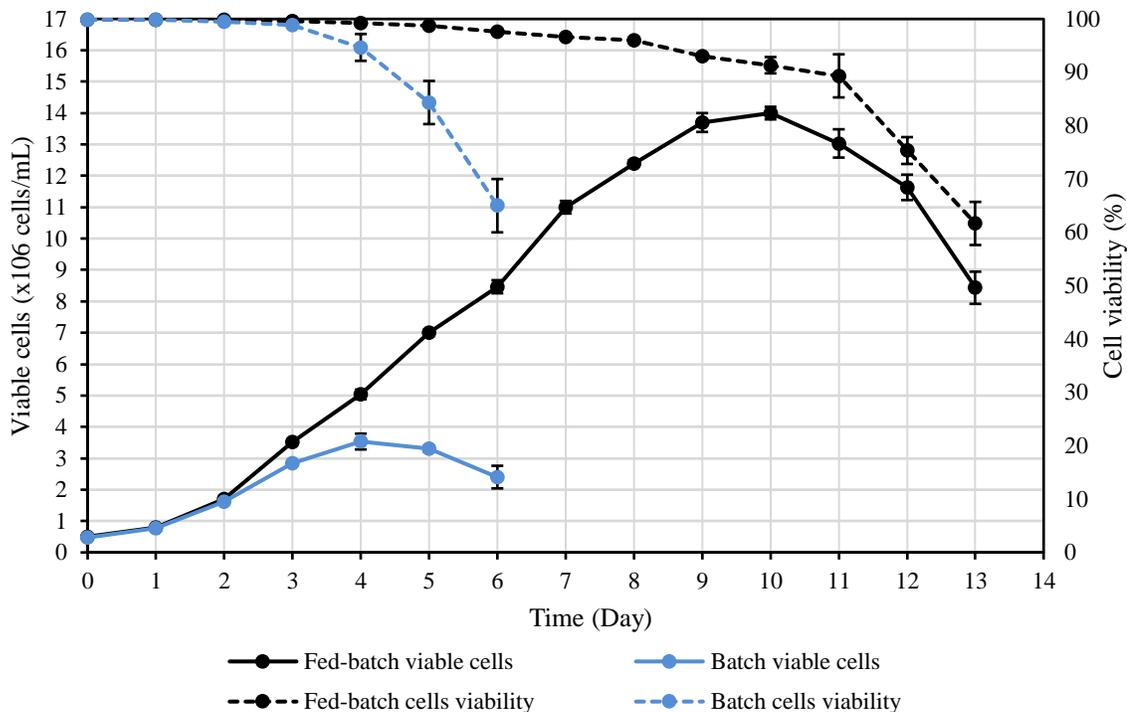
Figure 23. Growth profile for fed-batch culture using 100% SFM4CHO medium with Cell Boost 7a-without glucose/7b and batch culture using 100% SFM4CHO medium.
