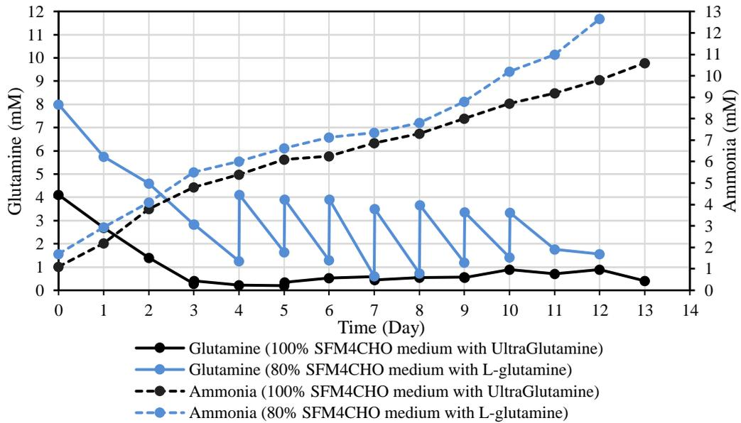
Figure 22. Glutamine and ammonia profile for fed-batch cultures using 100% SFM4CHO medium with UltraGlutamine and 80% SFM4CHO medium with L-glutamine.
