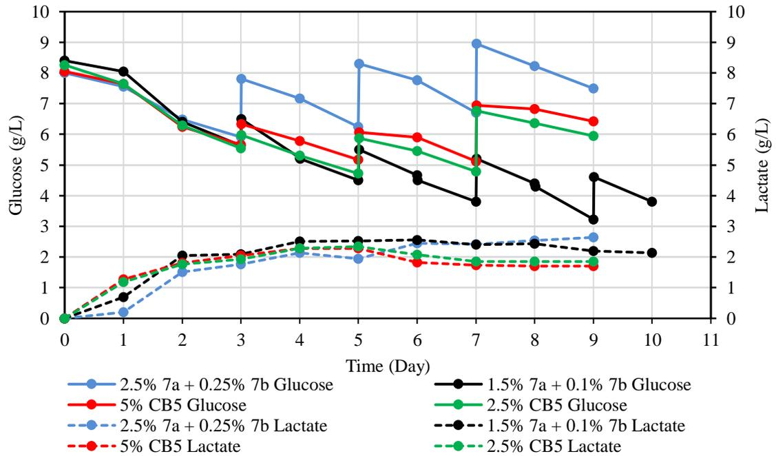
Figure 12. Glucose and lactate concentration profile for fed-batch culture using cell supplements 7a/7b or CB5 every other-day.
