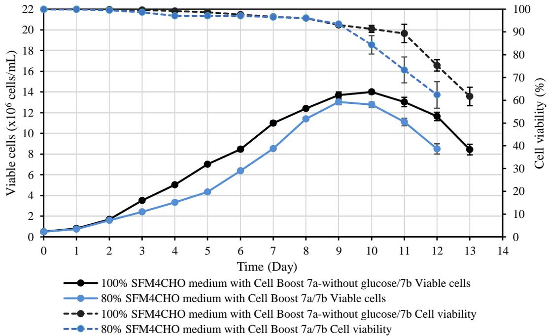
Figure 20. Growth profile for fed-batch cultures using 100% SFM4CHO medium with Cell Boost 7a-without glucose/7b and 80% SFM4CHO medium with Cell Boost 7a/7b.
