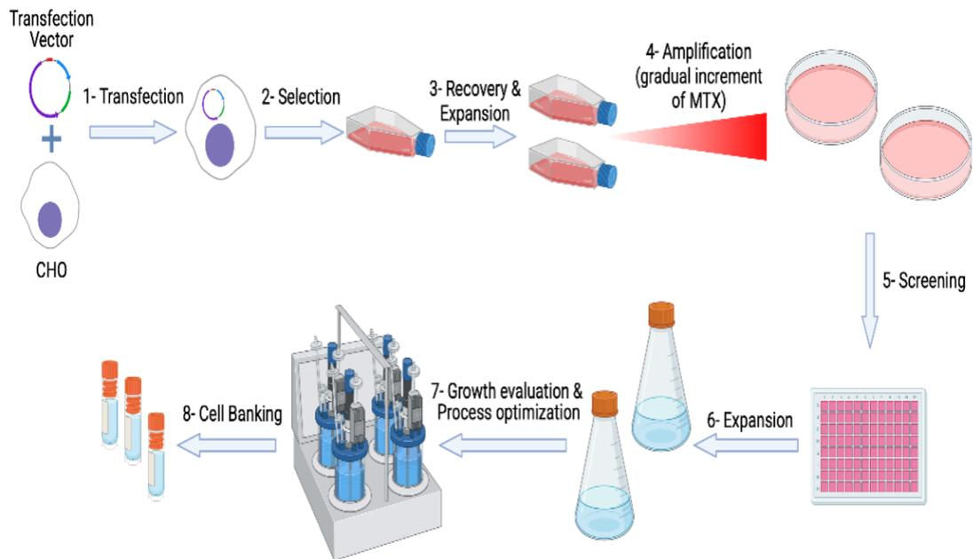
Figure 1. A Schematic of steps of CHO cell line development for recombinant protein production.
