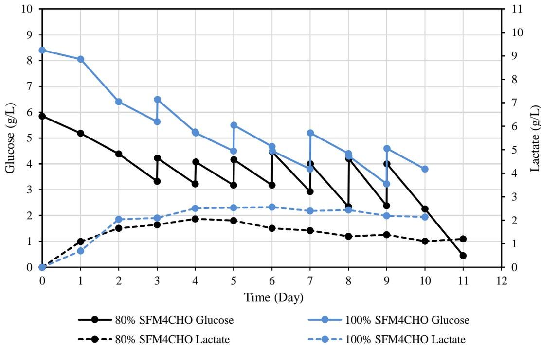
Figure 15. Glucose and lactate concentration profile for fed-batch culture using 1.5%:0.1% Cell Boost 7a/7b every other day with 100% and 80% SFM4CHO medium.
