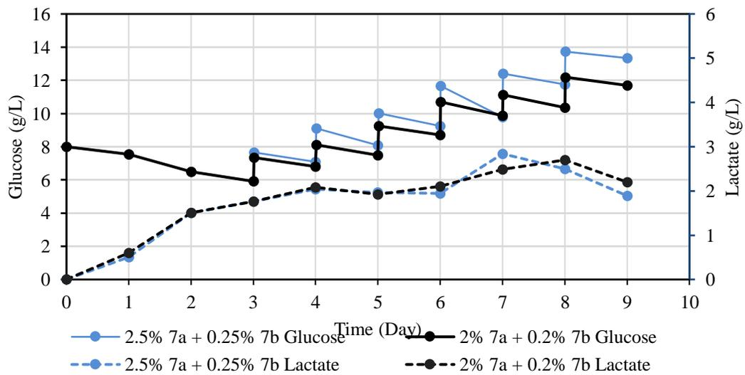
Figure 10. Glucose and lactate concentration profile for fed-batch culture using Cell boost 7a and 7b on day 3 every day.
