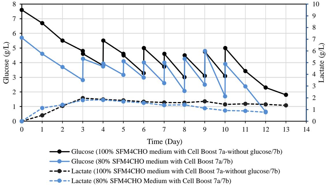
Figure 21. Glucose and lactate profile for fed-batch cultures using 100% SFM4CHO medium with Cell Boost 7a-without glucose/7b and 80% SFM4CHO medium with Cell Boost 7a/7b.
