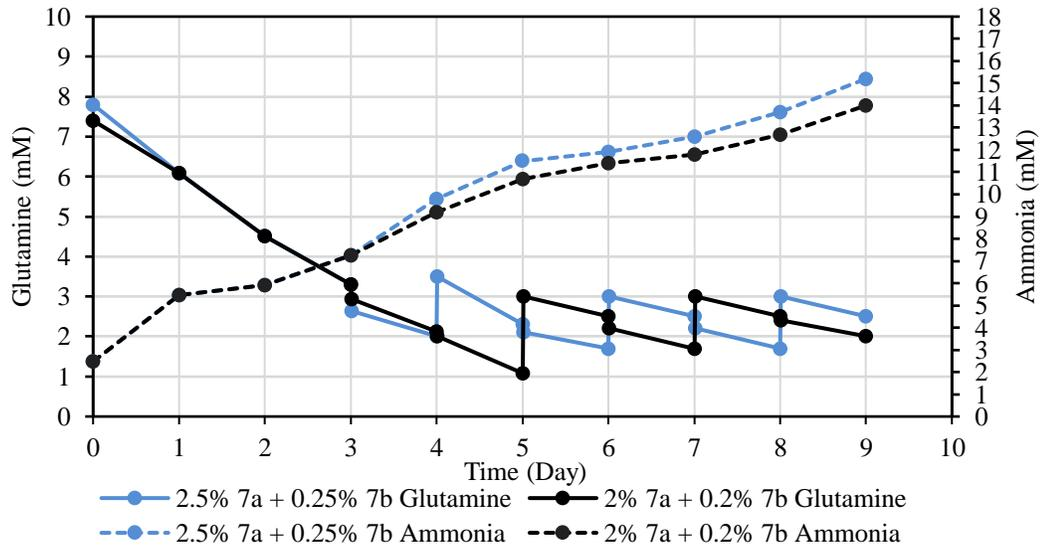
Figure 9. Glutamine and ammonia concentration profile for fed-batch culture using Cell boost 7a and 7b on day 3 every day.
