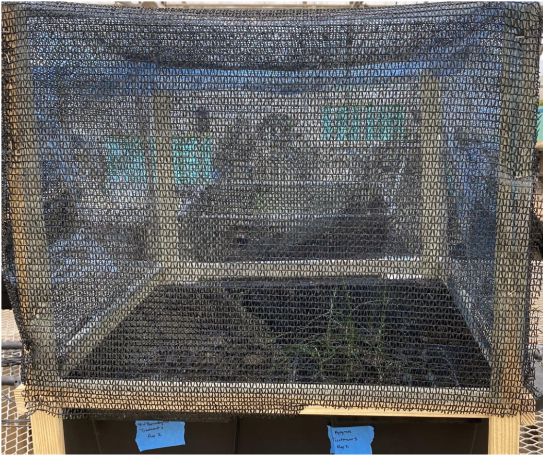
Illustration B.2. Overview of a shade structure to investigate the response of bermudagrass and perennial ryegrass to a reduction in R:FR ratio combined with a reduction in PPF with a photoselective blue polyester gel filter and 40% black shade net.
