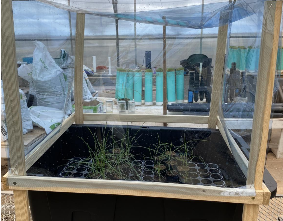
Illustration B.1. Overview of a shade structure to investigate the response of bermudagrass and perennial ryegrass to a reduction in R:FR ratio with minimal PPF reduction with a photoselective blue polyester gel filter (Lee Filters, Burbank, CA).
