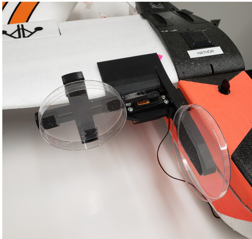
Figure 57: Leading Edge Wing Mount
