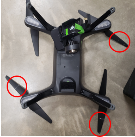
Figure 61: Chalk traces on propellers
