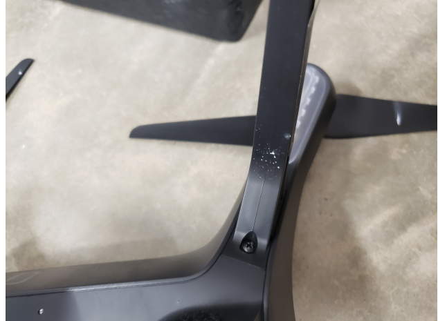
Figure 62: Chalk particles on landing gear
