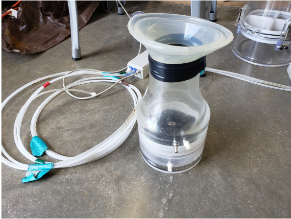
Figure 27: Dolphin flow meter
