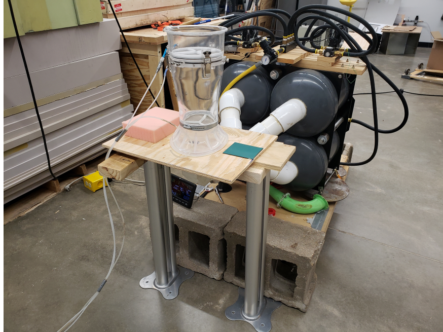
Figure 29: Flow meter test setup
