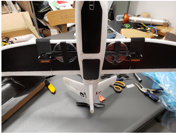
Figure 58: Bottom Wing Mount
