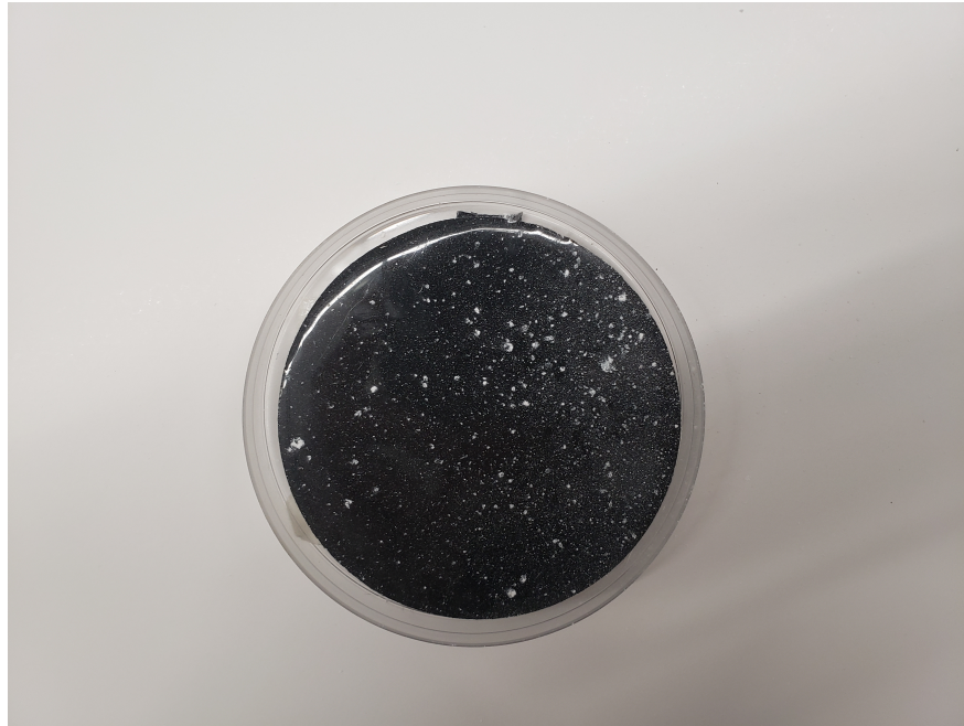
Figure 50: Open Nozzle chalk test (3ft)
