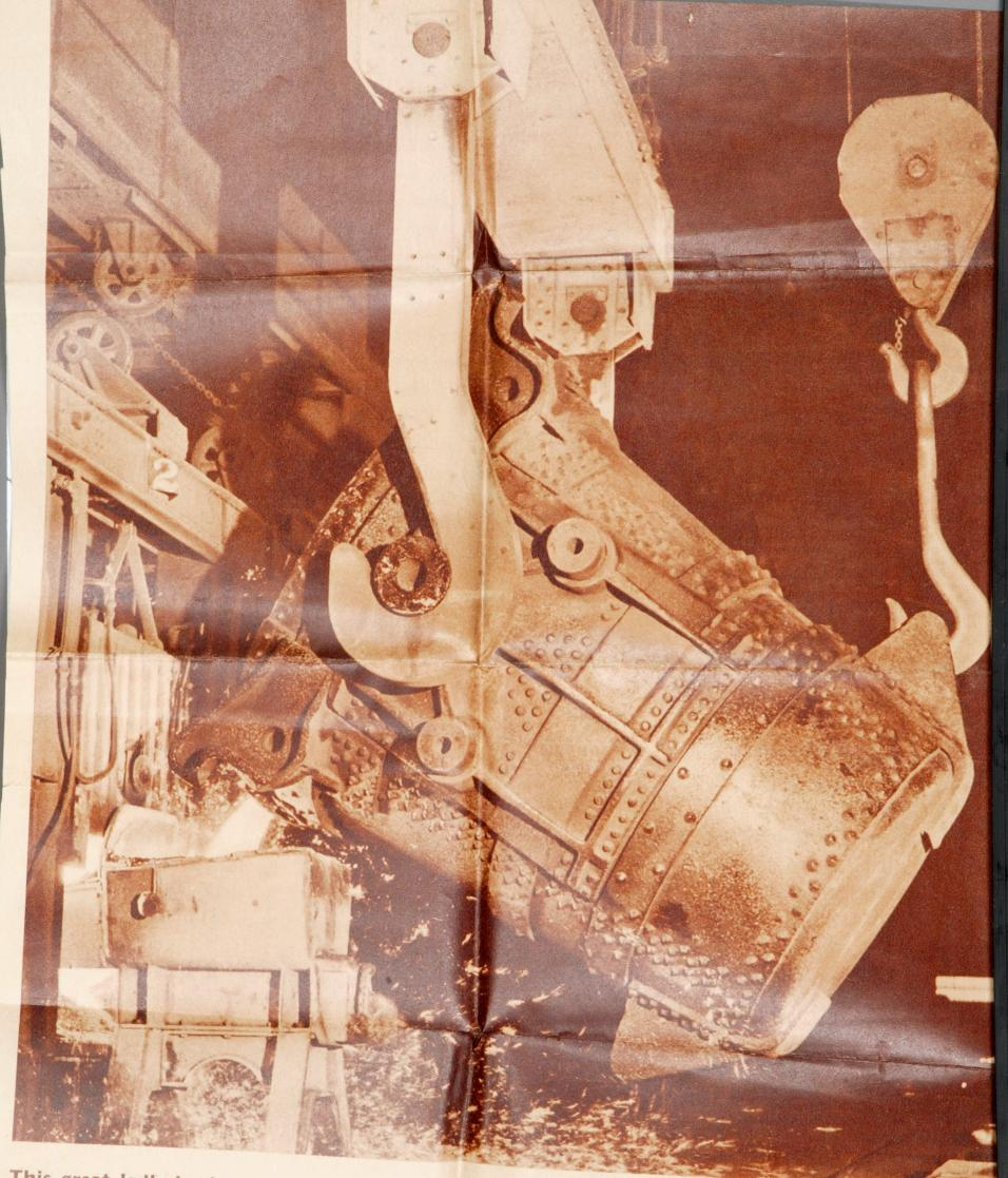
This great ladle is charging an open hearth furnace with 52 percent scrap and 48 percent molten iron. After about 13 hours of intense heat the charge will become steel.
