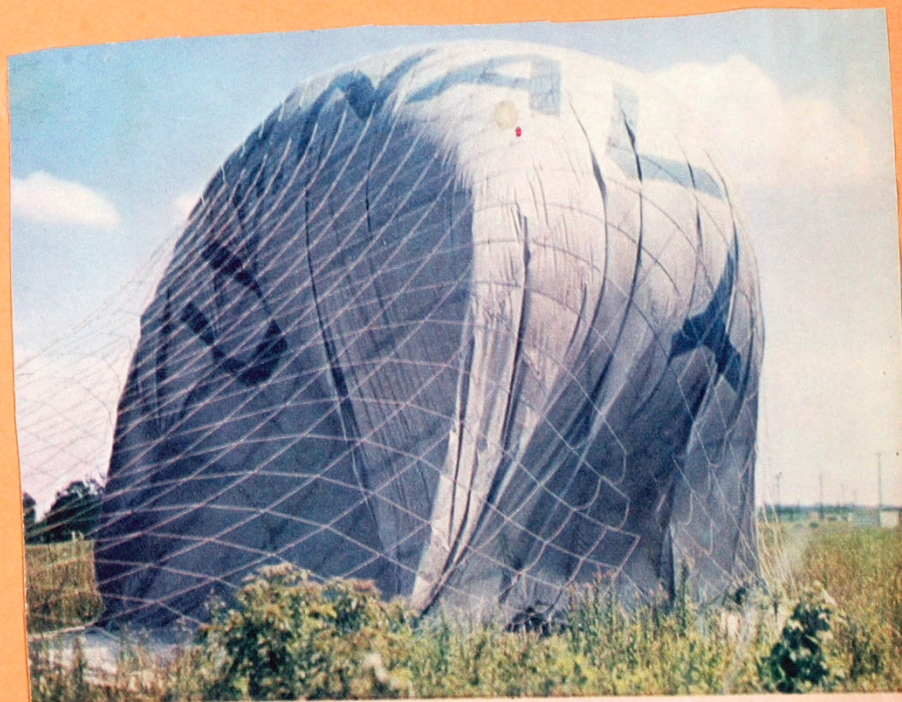
Three and a half hours later the pilot chooses a landing spot and, as the balloon lands, pulls a rip-cord opening the ripping panel at the side to release the gas. In a moment the bag above will be completely collapsed
