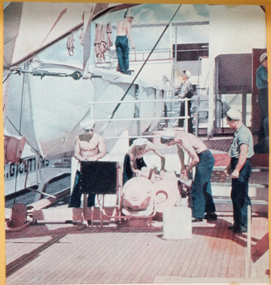
Apprentices on training ship American Seaman working around davit winches. Trainees quickly learn that all equipment must be kept in first-class condition
