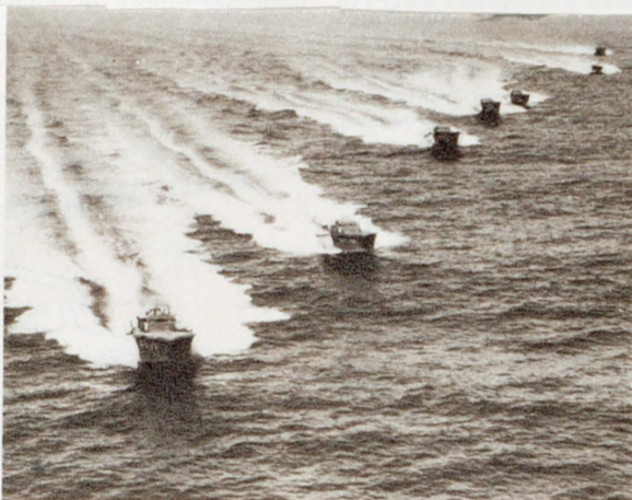
A Squadron of snarling PT boats race down the sea-board in echelon formation. Each of these Patrol Torpedo boats houses three 1350 h.p. Packard marine engines. Evidence of their tremendous power is clearly written in those white wakes and plumes of spray.
