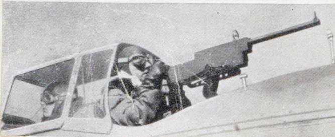
The U. S. is following Britain in placing camera machine guns in actual fighters, to record fights
