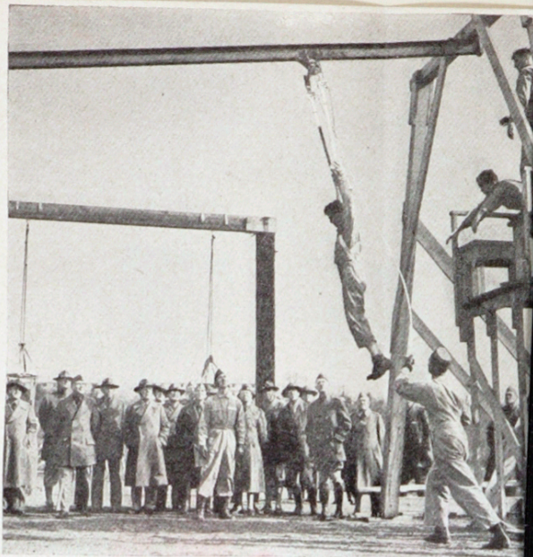
2 With this apparatus, which imitates the sideways drift of a landing 'chute, they learn to yank the suspension lines to lessen the shock
