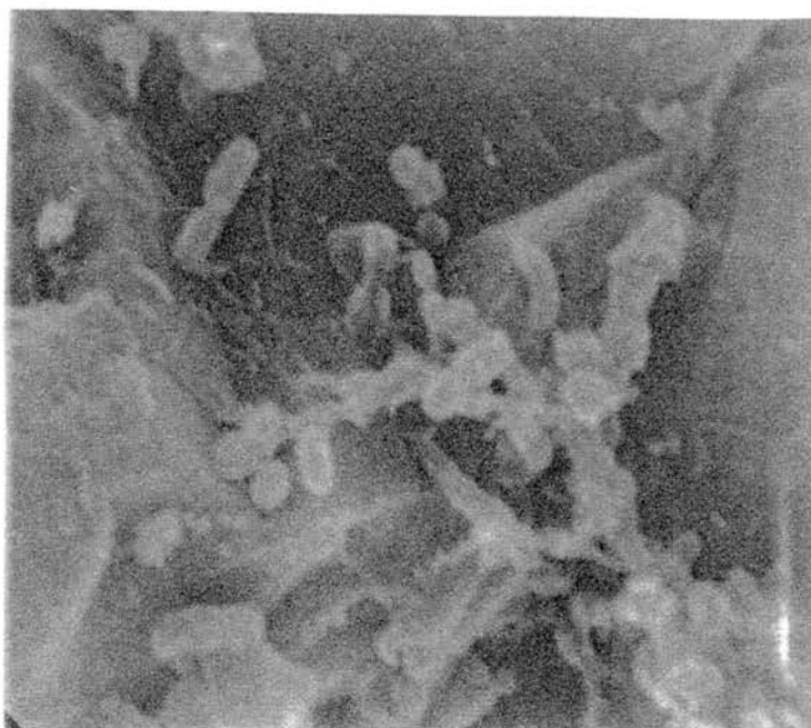
Figure 152. The population of the GAC immobilized cells shown in GAC column #4 after shock load (16,000 X).
