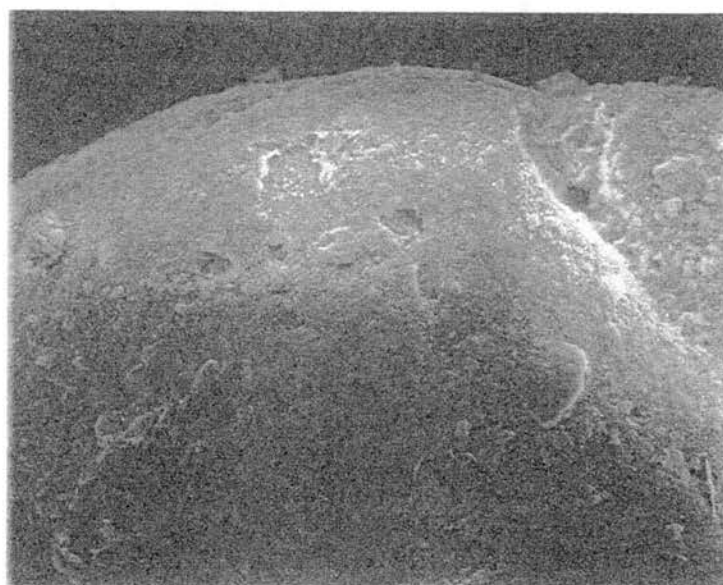
Figure 136. The outer surface of the PVA bead with immobilized bacteria 2 days old (72 X).
