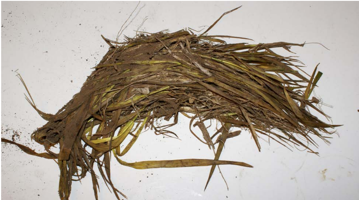
Fig 1. Improperly packaged wheat samples will rot during shipment and are inadequate for testing.
