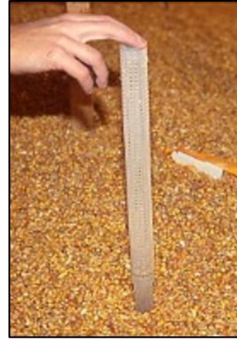
Fig. 4. Inserting probe trap
