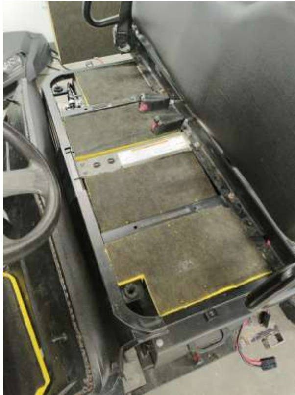
Figure 7: Insulation between compartment and seat
