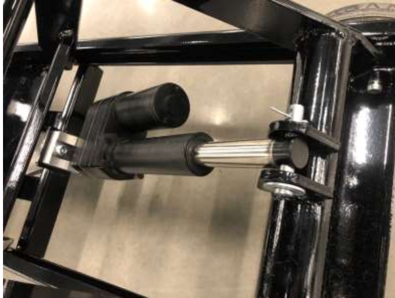
Figure 21: An electric linear actuator replaced the original hydraulic lifting system to increase ease of use and reduce weight.
