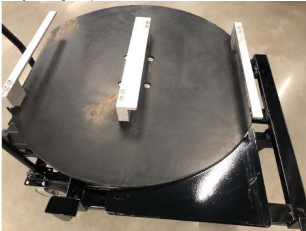
Figure 22: A rotating tabletop was added to the cart to enable simultaneous battery module exchanges.
