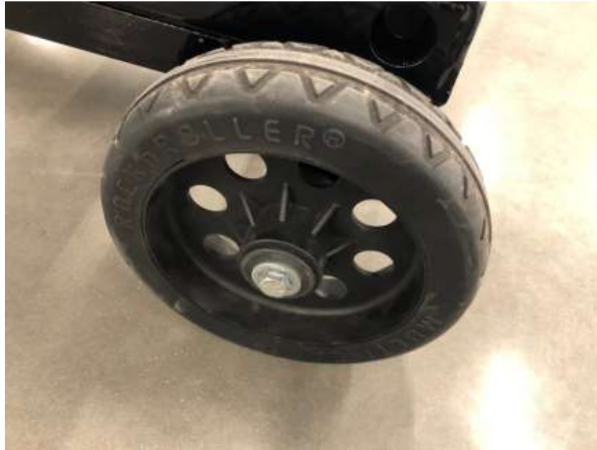
Figure 23: Larger diameter wheels with all-terrain tread patterns were added to increase terrain access during UTV battery exchanges.
