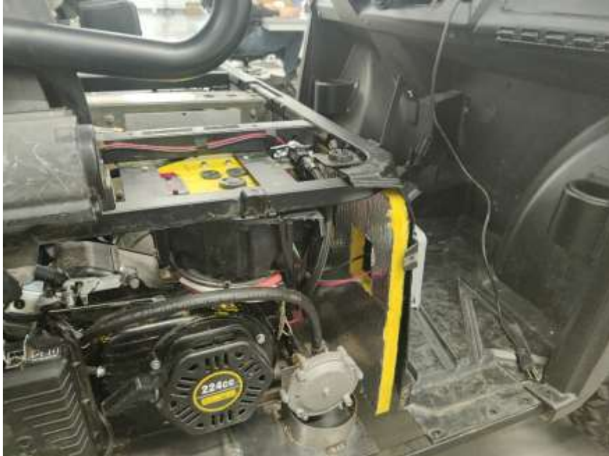
Figure 8: Insulation between footwell and compartment
