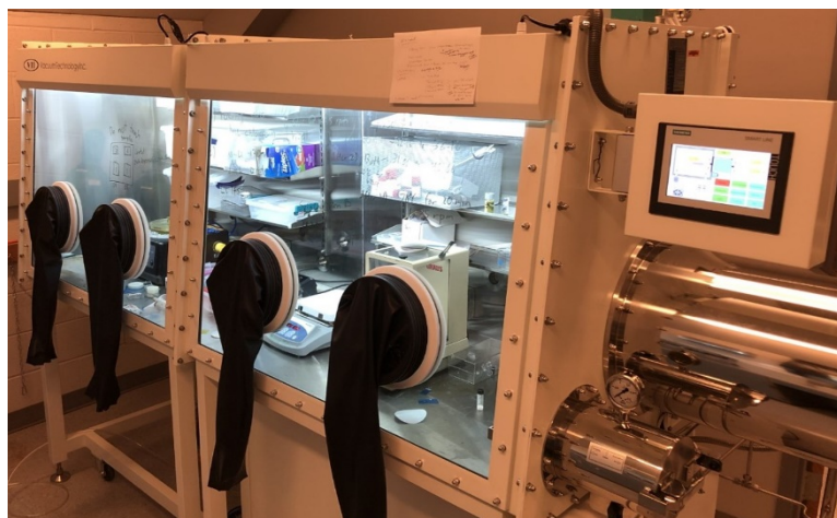
Figure 11: Photo of double glove box with spin-coater and heater for air sensitive synthesis of the hybrid halide perovskite and hole transport layers.
