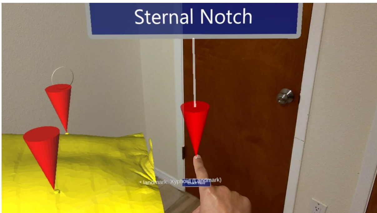
Figure 22: Upon recognition of “Check Here” feature the highlighted landmark-pin is placed at the tip of the index finger of the operator. Upon placement, the pin is no longer highlighted. Upon touching any of the pins, a tooltip pops up showing the name of the destination anatomic location. This pin is supposed to be placed at sternal notch.
