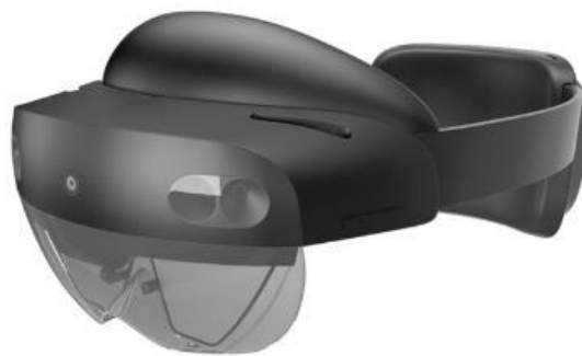
Figure 5: Microsoft HoloLens-2 [16] an optical see-through mixed reality headset. User always has direct natural view of the world. The AR contents are projected to the user's eyes via lasers.
