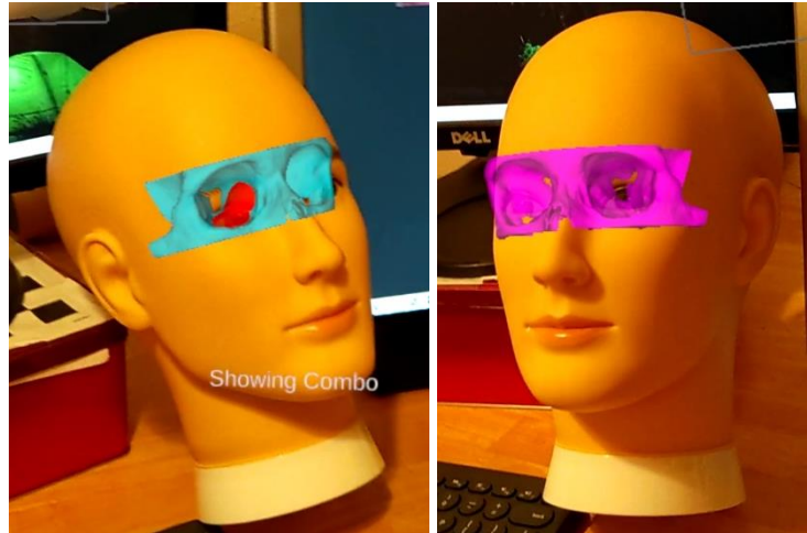
Figure 48: In the first image a red “combo” plate is shown. The objective of the surgery is to place the actual physical “combo” plate at same pose as this red hologram. The mirror of the “before” 3D model is shown in the second image. This “after” 3D model represents how the bones segment should look like if the reconstructive surgery was performed successfully.
