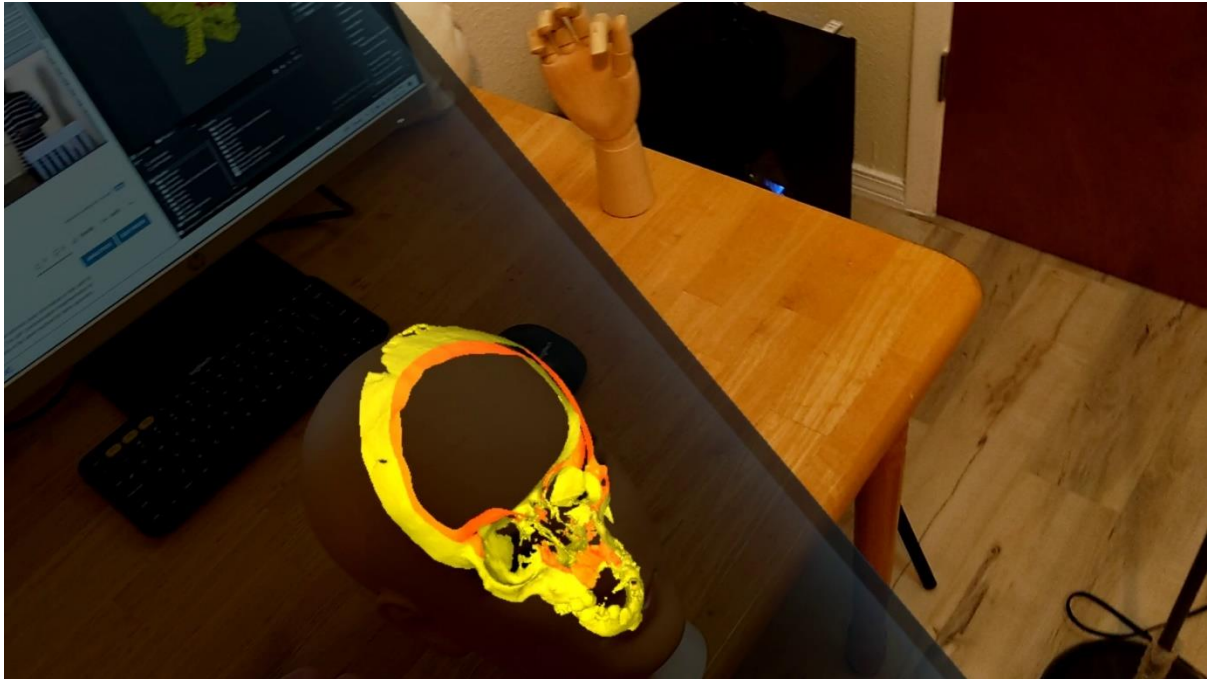
Figure 34: A vertical dissection is created by placing the slicing-plane at a tilted position.
