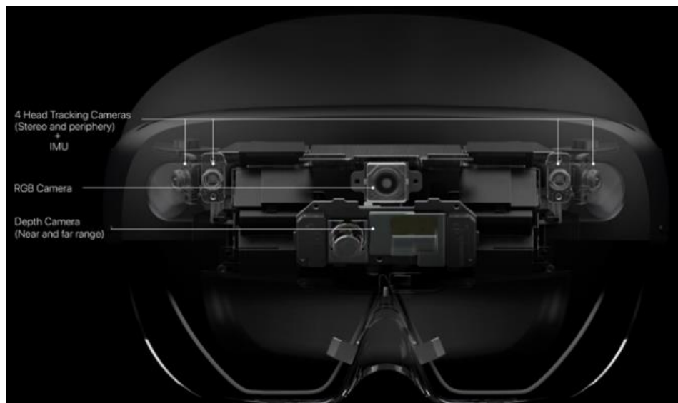
Figure 17: Outline of different sensors of HoloLens-2 [30]. IntraOpVSP currently only use the RGB camera, also known as the photo-video (PV) camera [31].
