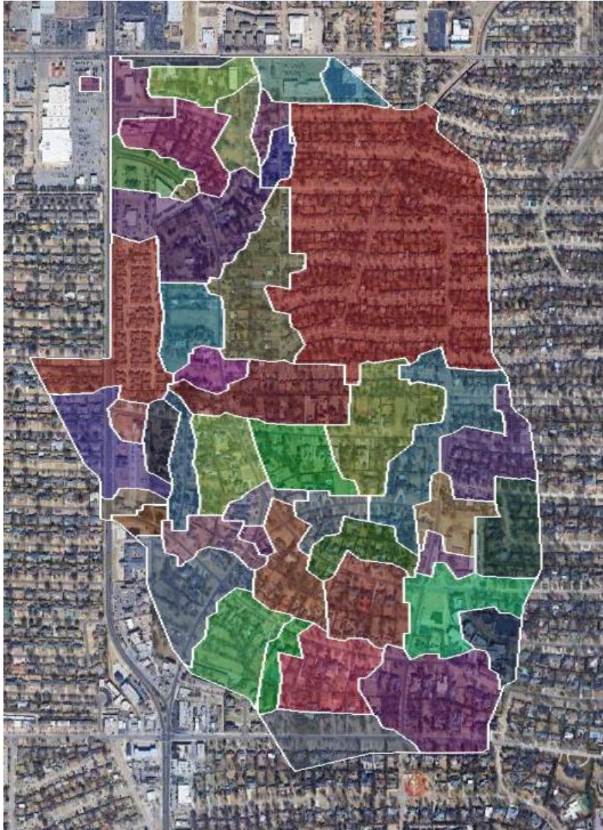
Figure 15. Subwatershed division for Sunnymead in Oklahoma City, Oklahoma. Base map: (Google Earth, 2021)
