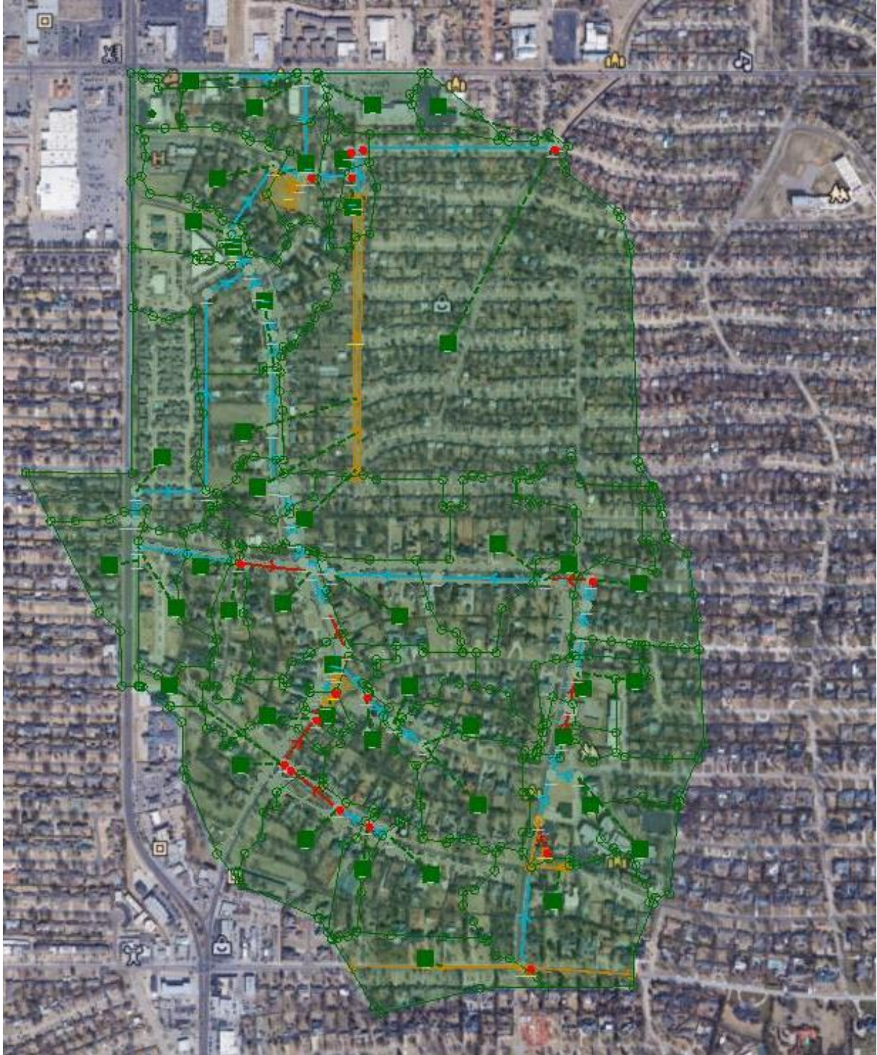
Figure 40. Proposed LID $4M open-lot bioretention + pervious concrete gutter and street system in Sunnymeade, Oklahoma City, Oklahoma for a 10-year storm event. Areas in blue are the existing storm sewer system, areas in red represent flooding in the system, areas in orange are the LID system (Google Earth 2021; Innovyze, 2021)
