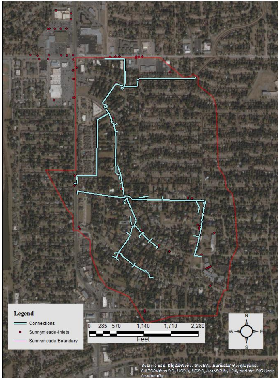
Figure 14. Existing storm sewer system and inlets for Sunnymead in Oklahoma City, Oklahoma. Base map: (ESRI, 2021)
