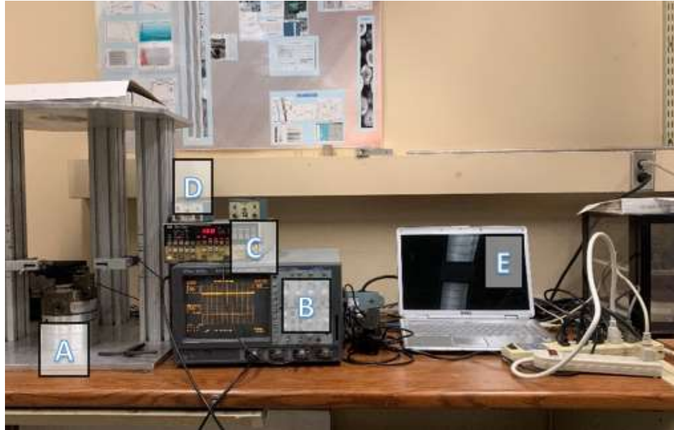
Figure 4-1. Circumferential Velocity Analysis (CVA) set-up. It includes A) the motor that rotates the base, B) The oscilloscope which digitizes the acoustic wave, C) the signal generator which sends the pulse to the excitation transducer, D) Amplifiers, E) Computer.
