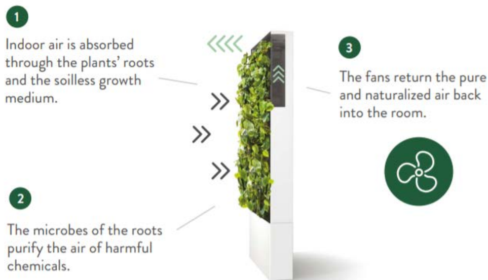
Figure 16 Naava active living wall air purifying process (Naava, n.d.)
