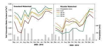
Figure 3. Monthly average of soil water content at four soil depths in a grassland watershed and a redcedar watershed.
