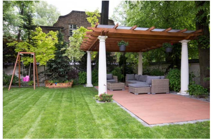
Figure 5. Combining turfgrass and water-pervious hardscapes, like pavers, can enhance the landscape, while reducing irrigation demand and managing run-off.
