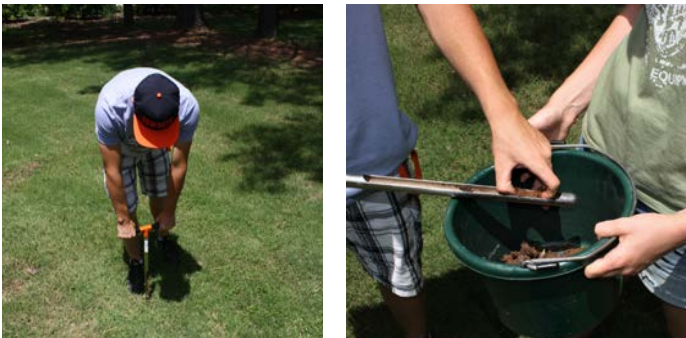
Figure 3. Use a soil probe or shovel to sample from 15 to 20 random locations and mix in a clean bucket.
