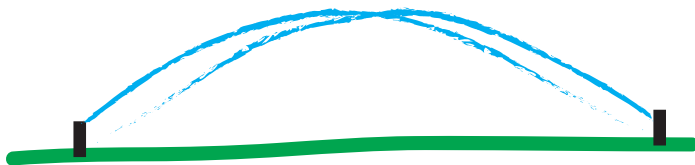
Figure 10. Head-to-head coverage ensures uniform water distribution.
