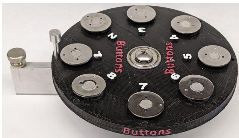
Figure 3.1 – 3D printed 8-position button carousel.
