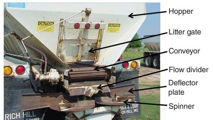
Figure 1. Working Parts of a Typical Litter Spreader Truck.
