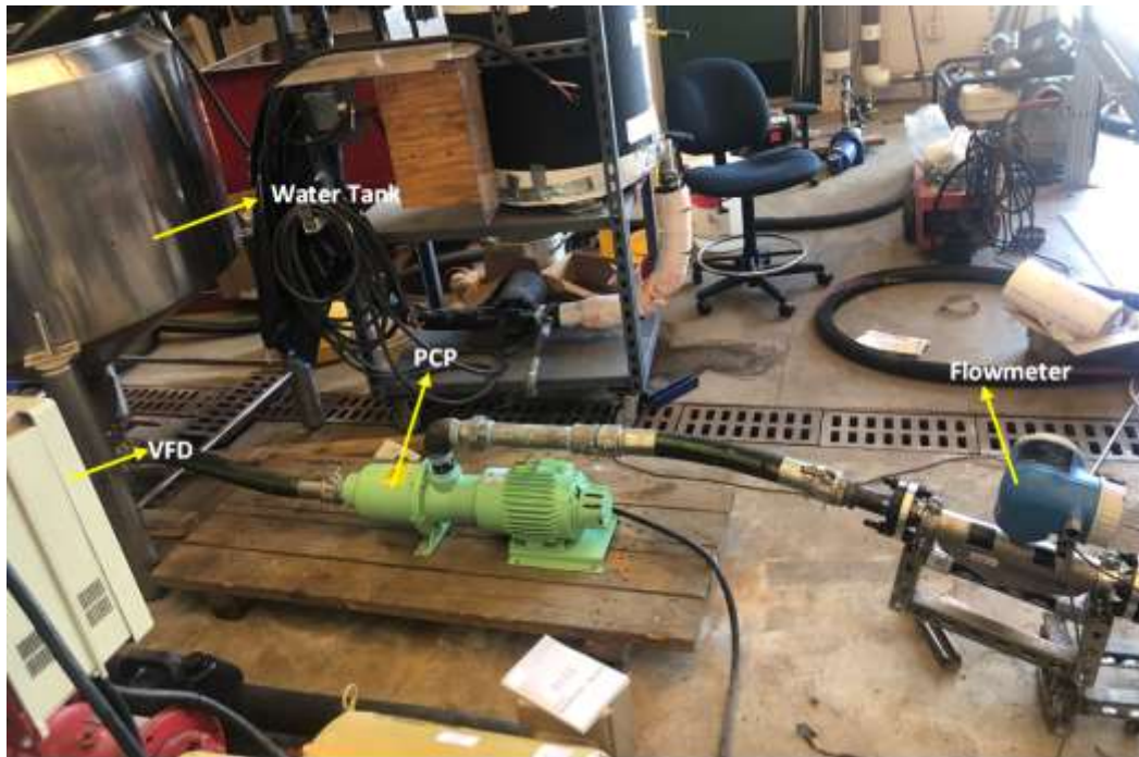
Figure 3.6. Water inlet line
