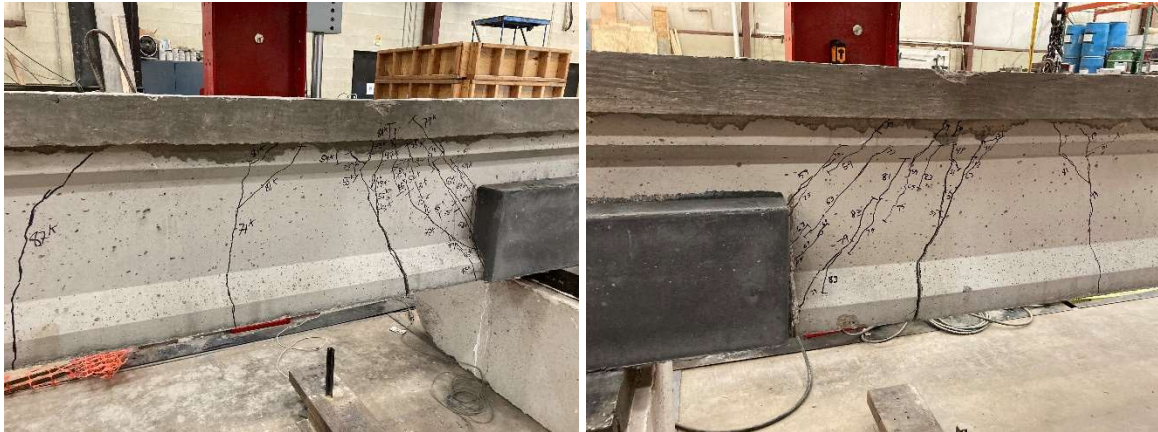
Figure 4.27: UHPC-2 Girder after Test with SW Side (Left) and SE Side (Right)
