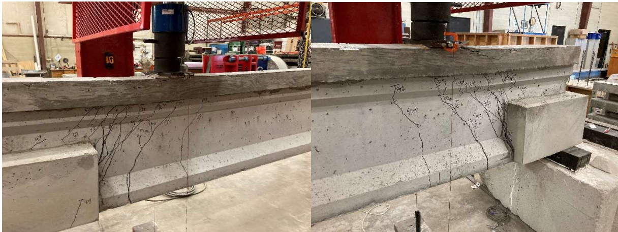
Figure 4.13: FR-SCC-1 Girder after Test with SE Side (Left) and SW Side (Right)
