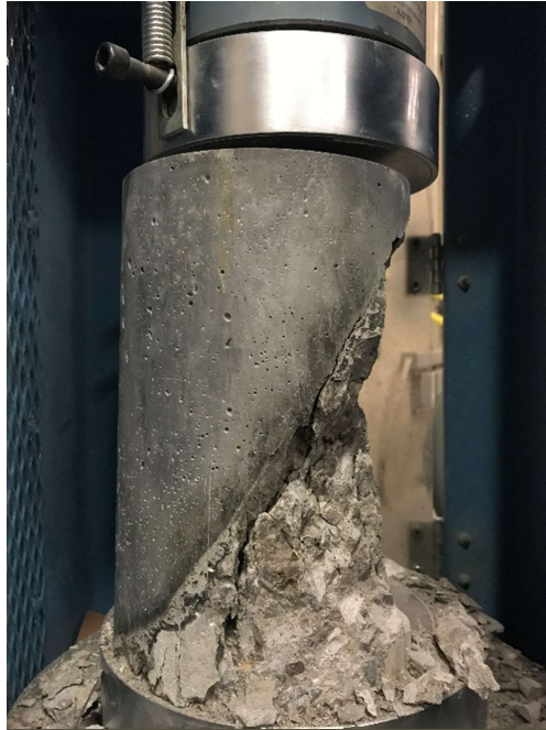
Figure 4.1: Specimen after Slant Shear Test
