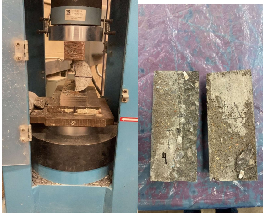
Figure 3.16: Specimen Break at Maximum Stress (Left) and Specimen Separated in Half After Test (Right)
