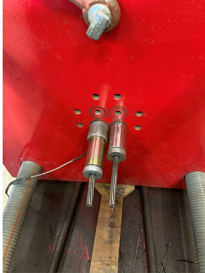
Figure 3.5: Position of Mark, Load Cell, and Chuck in Preparation for Pre-tensioning
