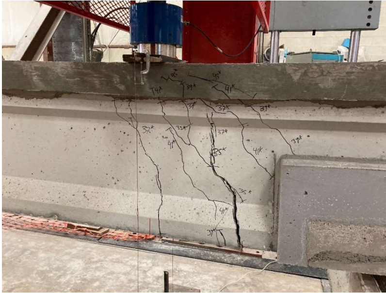
Figure 4.3: MALP-1 Girder after Test
