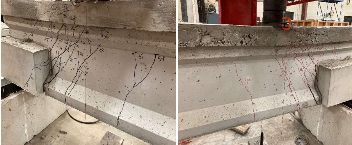
Figure 4.20: FR-SCC-3 Girder after Test with SE Side (Left) and SW Side (Right)
