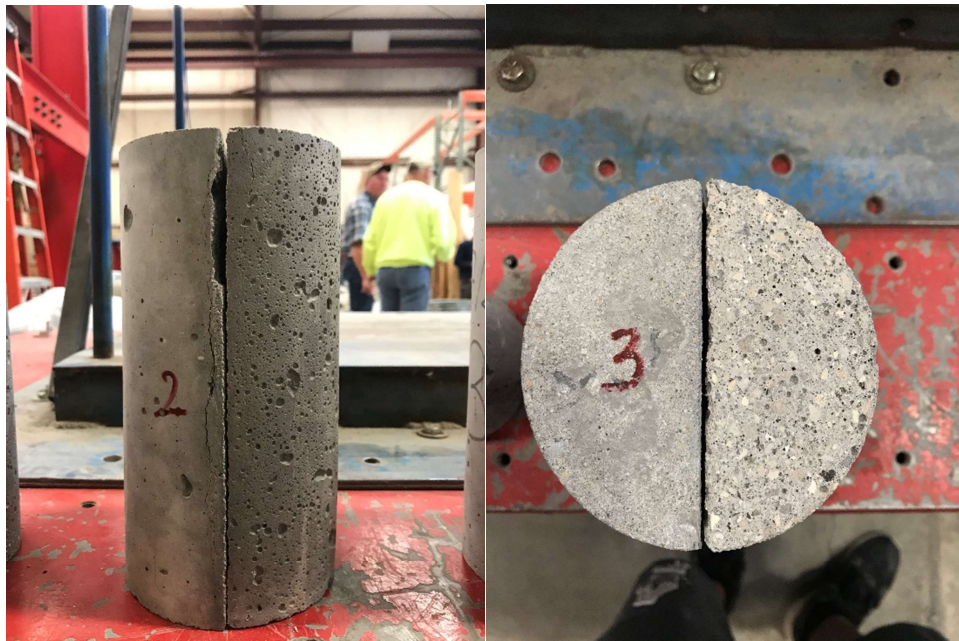
Figure 4.2: Specimen after Splitting Tensile Test at Side View (Left) and Top View (Right)
