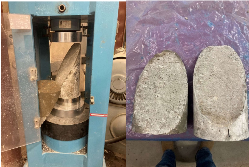
Figure 3.19: Specimen Break at Maximum Stress (Left) and Specimen Separated at the Inclined Surface (Right)
