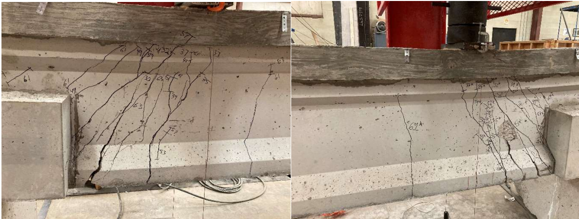
Figure 4.17: FR-SCC-2 Girder after Test with SE Side (Left) and SW Side (Right)
