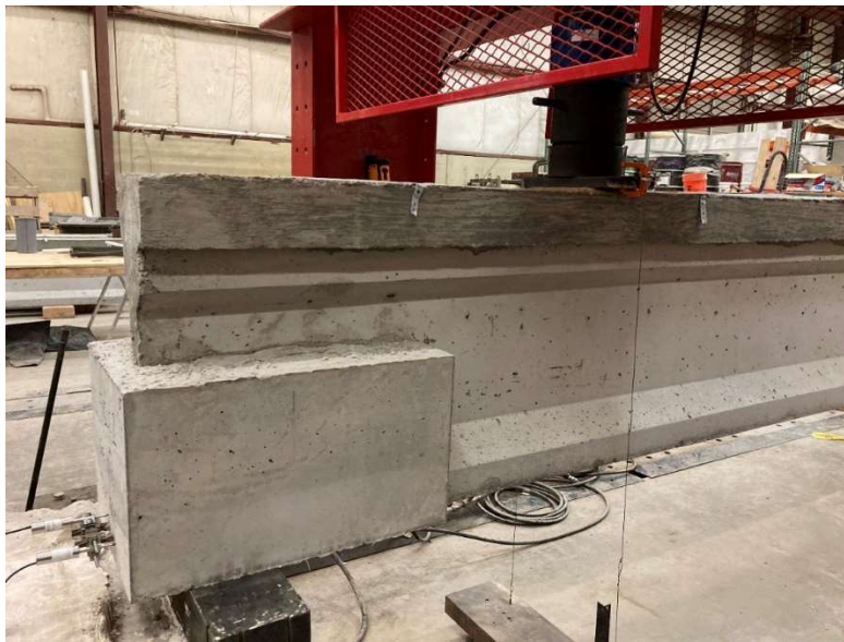
Figure 3.21: Finished FR-SCC Repaired Girder
