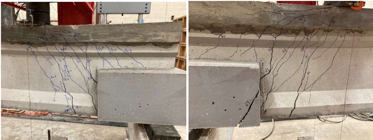
Figure 4.9: MALP-3 Girder after Test with SW Side (Left) and SE Side (Right)
