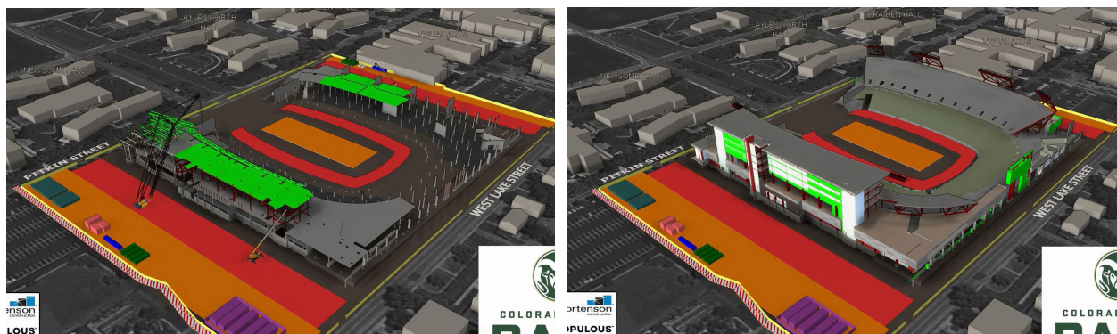
Screen shots of the animated 4D that was a powerful planning and logistics tool.
