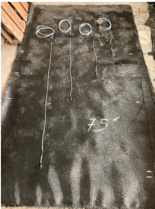
Figure 5 – Geotextile instrumentation; (Left) instrumented geotextile, (Right) WP connections to geotextiles
