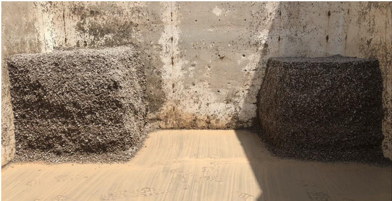
Figure 20 – Deconstructed test cubes; (Top) GRS Abutment Model #7 (yellow lines represent the measurement pattern), (Bottom) GRS Abutment Model #8
