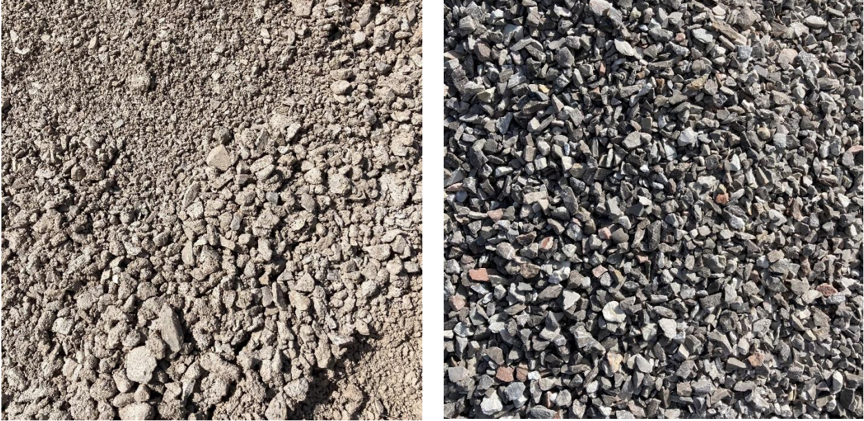
Figure 6 – Aggregate used for construction of GRS Abutment Models #7 and #8; (Left) ODOT Type A, (Right) 3/8” #2 Cover
