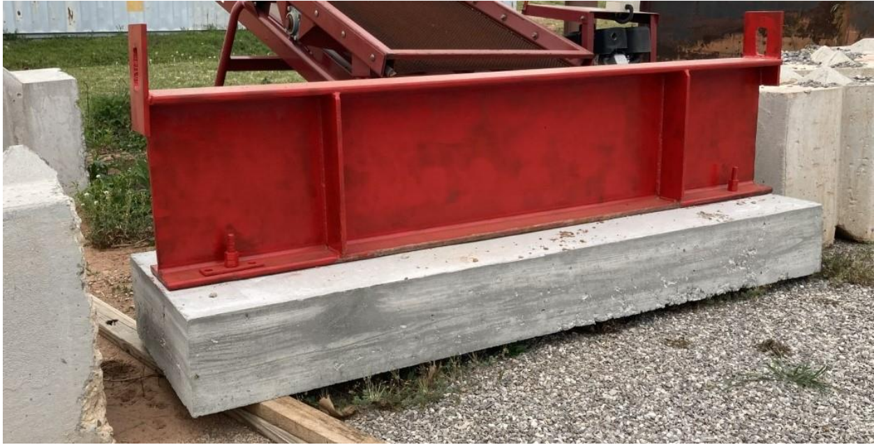
Figure 3 – Loading beam used in GRS Abutment Model #8
