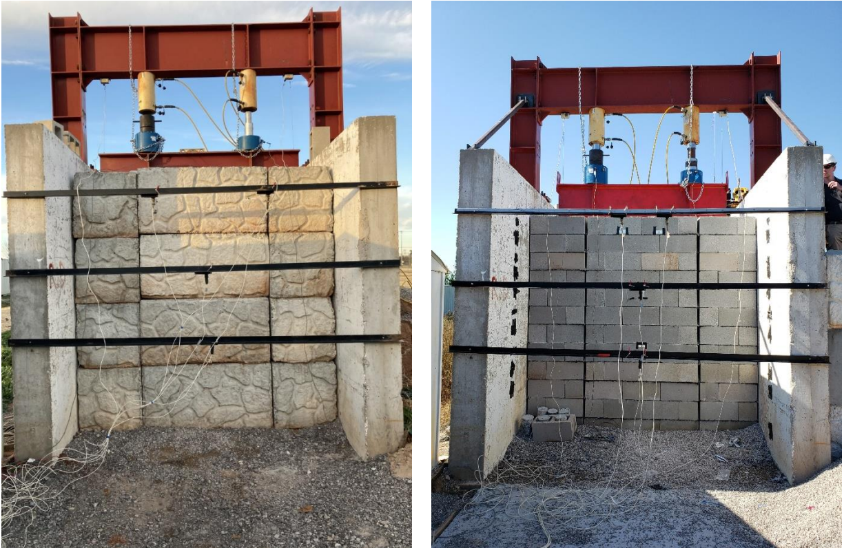
Figure 10 – GRS abutment models prior to surcharge loading; (Left) #7, (Right) #8
