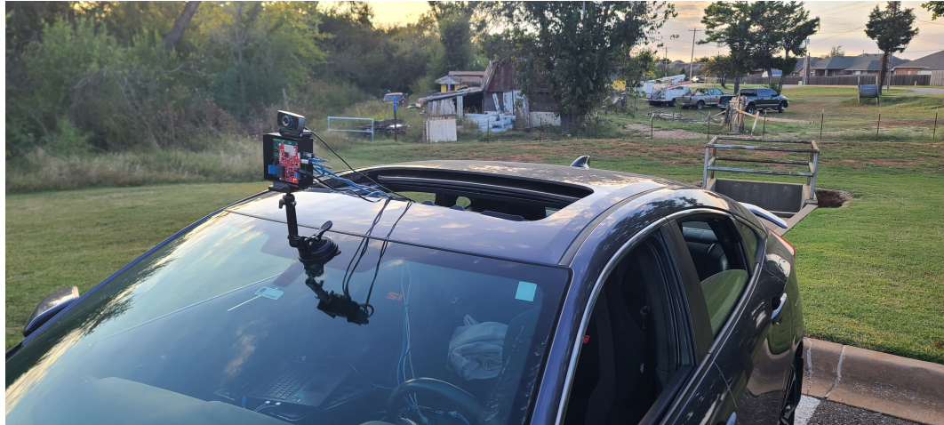
Figure 2.11: Using a suction cup phone mount with 3D printed mount, the full setup can be mounted to capture data while driving.
