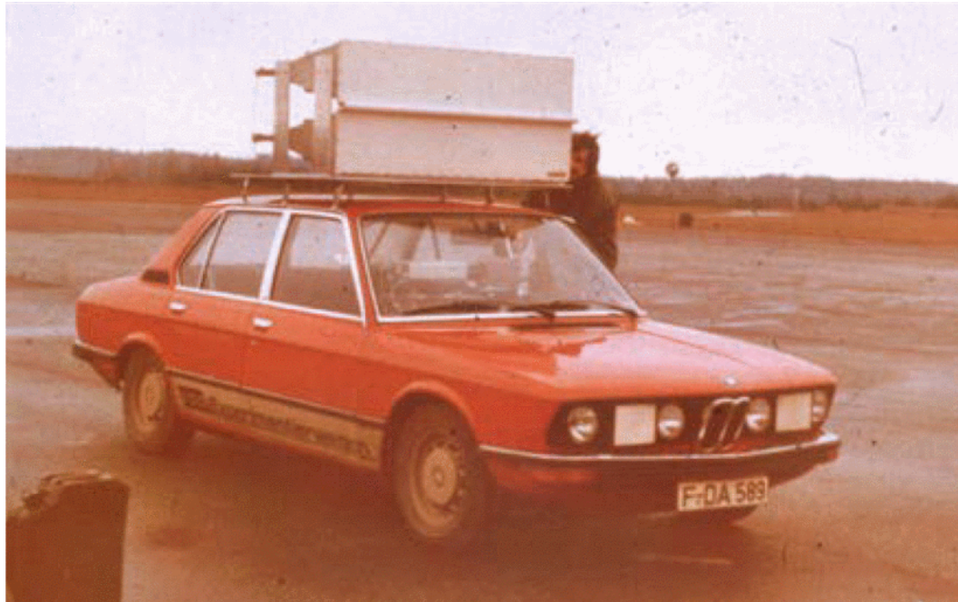
Figure 1.2: A 10GHz Horn system was mounted on top of the car, an example of the first automotive radar in the 1970s. Picture from the private collection of Holger H. Meinel[2].
