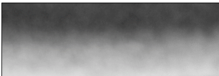
Figure 24: Thermographic threshold image of Set 2 sample, two different thickness of sample are visible, thicker (top), thinner (bottom)
