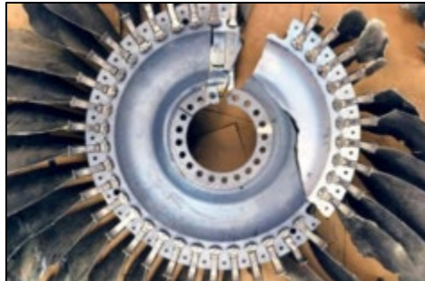
Figure 2: Failed fan disk from UA232 [22]
