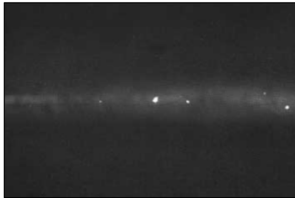
Figure 5: Radiographic image of a weld with inclusions (bright spots) [55]
