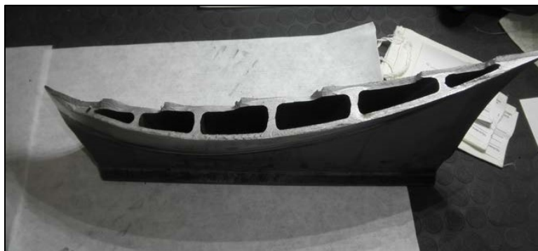
Figure 3: Fractured fan blade #11 from UA1175 [23]
