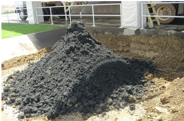
Figure 1. An example of biosolids after most water has been removed.
