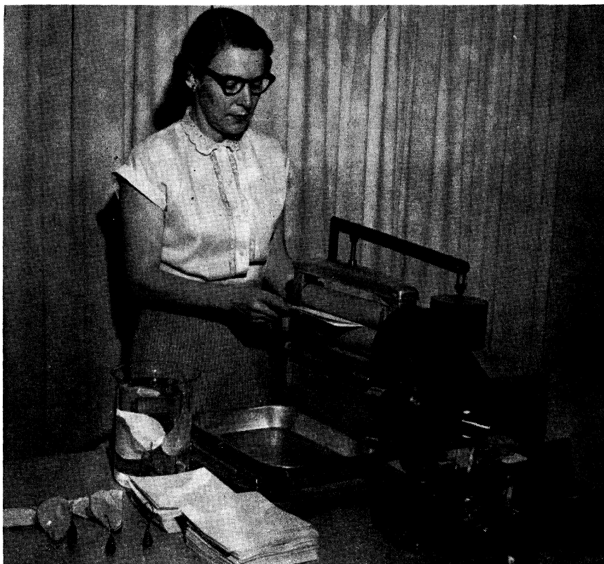
Figure 3. Apparatus used in measuring absorption by the static immersion method.
