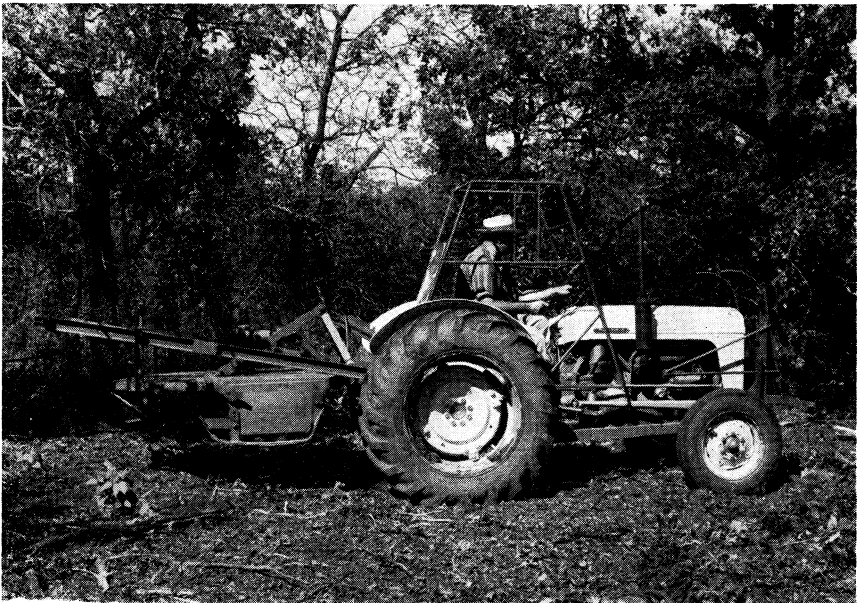
Fig. 4. Tractor mounted shredder unit.
