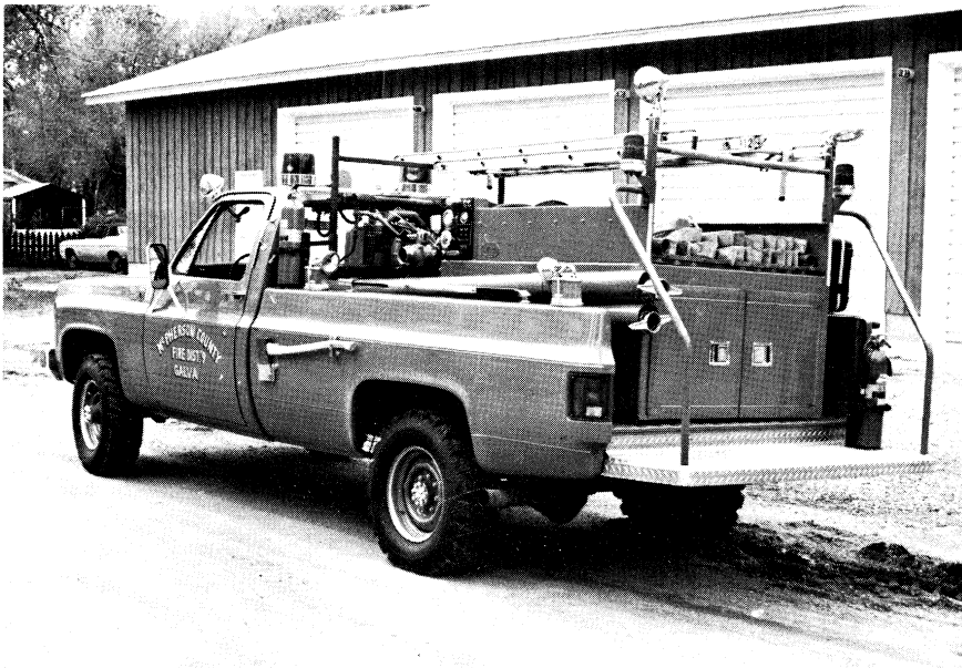
Figure 3. A pickup and slip-in unit ready for fire service use.
