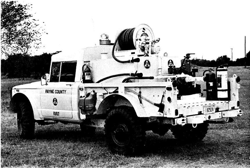
Figure 4. A military surplus vehicle converted for fire service use.
