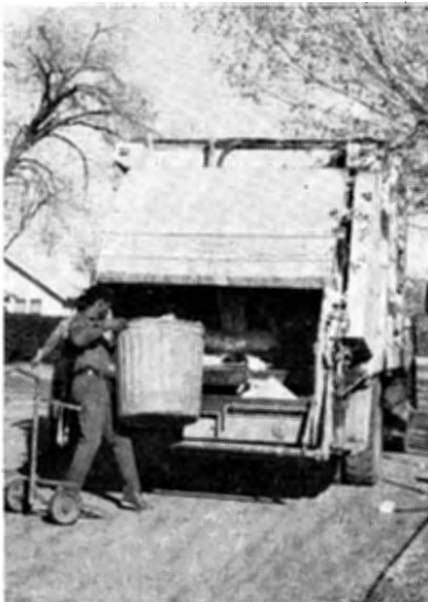
Figure 1. Typical solid waste collection compactor equipment, (left) rear loading and (right) front loading.
