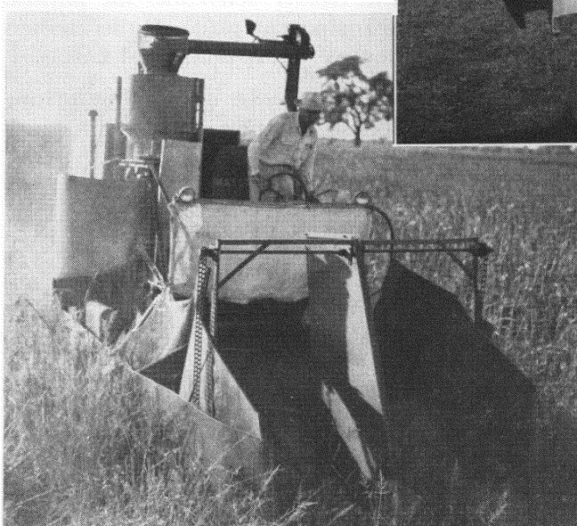
Fig. 8—Huller-cleaner mounted on a Massey-Harris castor bean combine.
