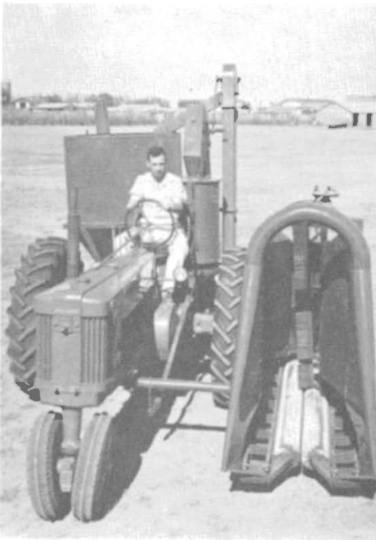
Fig. 6—Huller-cleaner (using centrifugal fan for cleaning) mounted on a USDA castor bean harvester.
