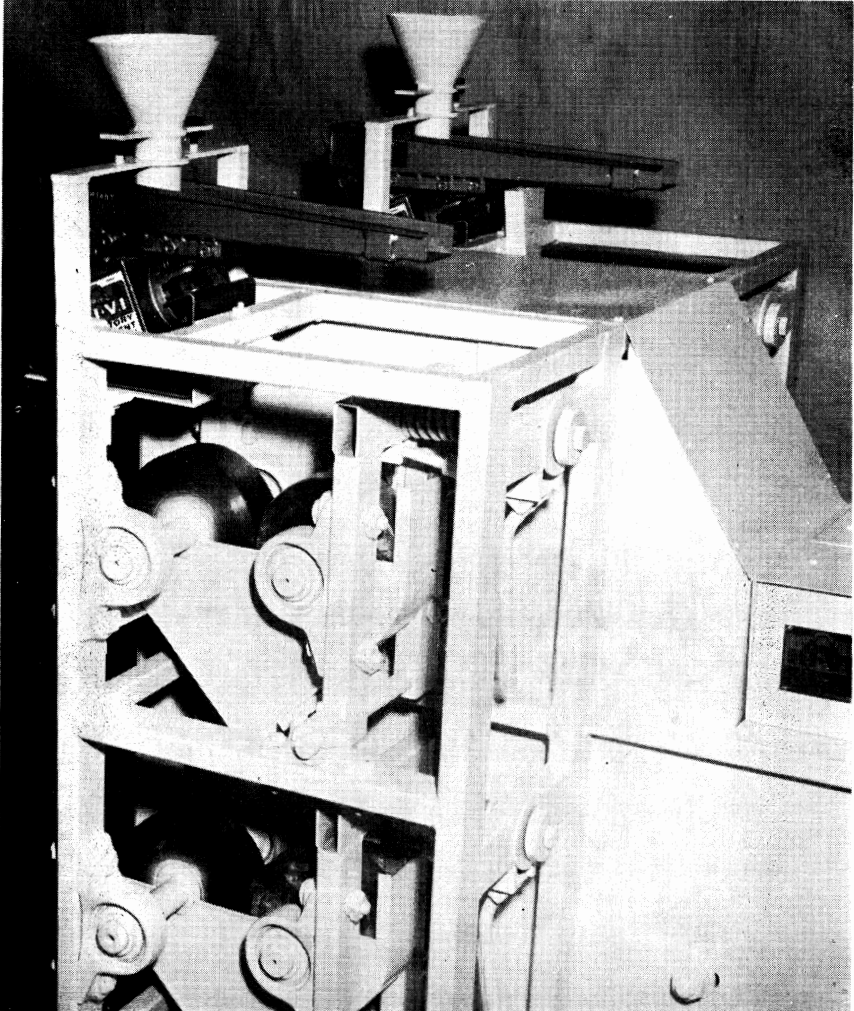
Figure 12. Break side of micro flour mill with roll covers and discharge spouts removed.
