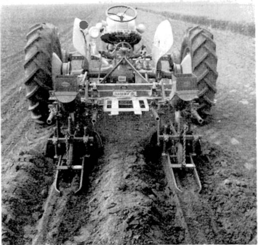
Figure 4.—Rear view of planter used to form new seedbed profile. Note the ditch produced by the disks on the side of the seedbed. The small rubber presswheel is shown just ahead of the open center covering drag.
