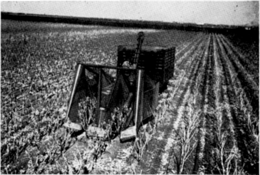
Figure 5. Oklahoma Agricultural Experiment Station and United States Department of Agriculture Stripper Type Castor Bean Harvester.
